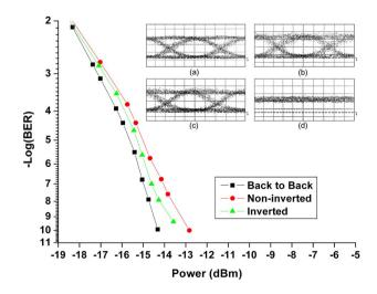
**Fig. 4** BER curves for noninverted and inverted wavelength conversions. Inset: Eye diagrams for (a) input signal, (b) noninverted converted signal, (c) inverted converted signal, and (d) FSK signal (the combined converted signals).
