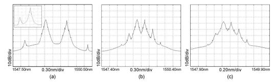
Fig. 5 Optical spectrum of the obtained FSK signal with tone spacing of (a) 0.8 nm, (b) 0.3 nm, and (c) 0.2 nm. Inset: The optical spectrum of demodulated FSK.
