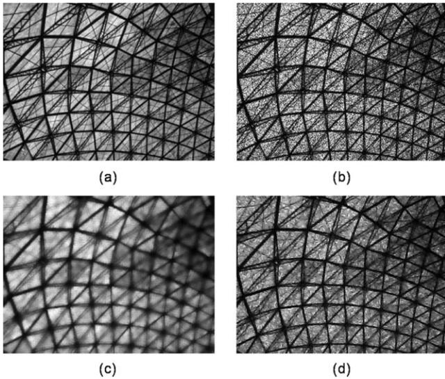
**Fig. 1** Roof images in experiment. (a) Original image. (b) Noisy image ( $\sigma = 15$ ). (c) Result with NL-means. (d) Result with NL-OMS.
