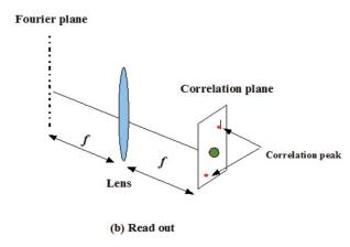
Fig. 7 Principle of the JTC (Ref. 7).
