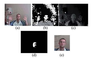
**Fig. 3** Example of head detection based on the (a) target image, (b) H component thresholding, (c) S component thresholding, and (d) head-detection results. (e) This figure shows the result from running the proposed method.
