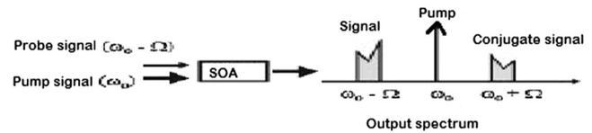
Fig. 3 Four-wave mixing in an SOA.
