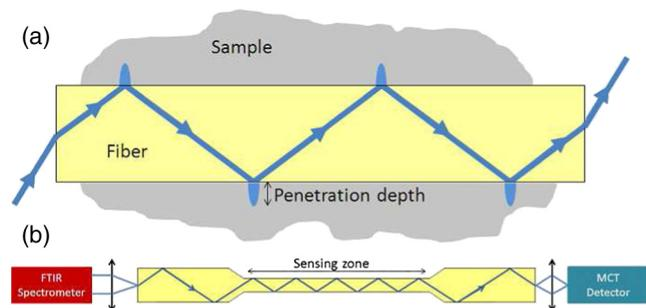
**Fig. 2** (a) Mechanism of fiber evanescent wave spectroscopy (FEWS). (b) General setup of FEWS and the scheme of a tapered fiber.<sup>4</sup>
