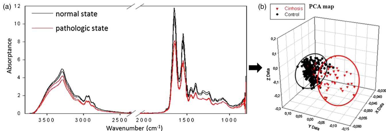
**Fig. 4** (a) FEWS spectrum of human serum with and without cirrhosis. (b) The corresponding principal component analysis (PCA) map.<sup>4,33</sup>
