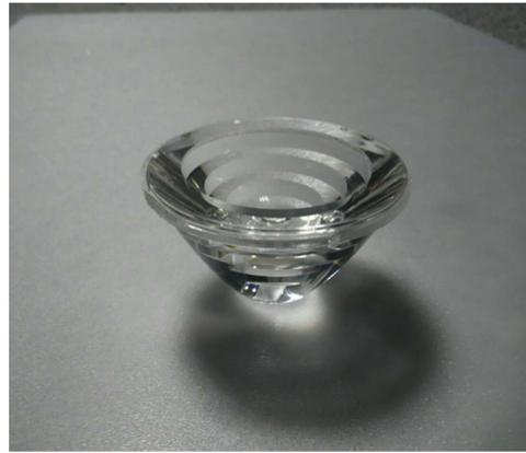
**Fig. 13** Lens with TIR surface designed with  $n_0 = 5.89$  mm and  $w_0 = 12$  mm. The contour was measured with the help of a contour graph (Taylor Hobson Talysurf PGI Dimension 3). The accuracy of the measure of profilometry is  $0.3 \mu\text{m}/\text{mm}$ .
