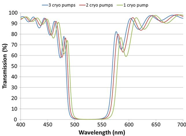
**Fig. 2** Transmission spectral scans of the HR coatings, taken at 45-deg AOI, P-pol. The HR bandwidths of each coating are 43, 43, and 45 nm for 3, 2, and 1 cryo pumps in operation, respectively. The HR bandwidths were measured over the interval where transmission <0.5%.
