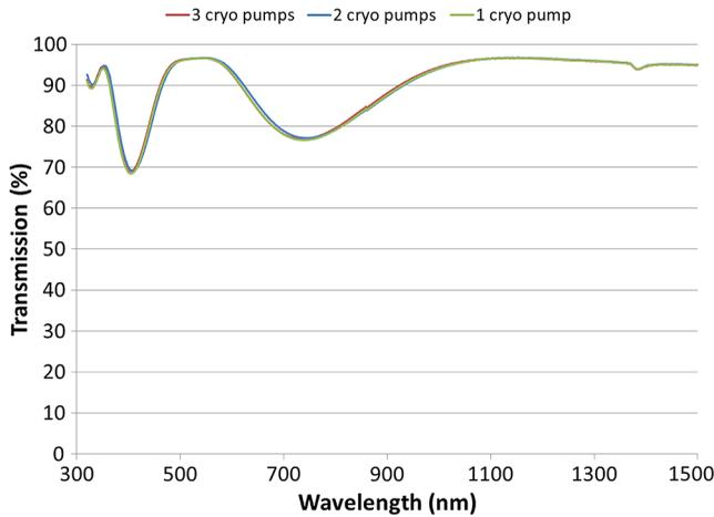
**Fig. 1** Transmission spectral scans of the AR coatings taken at 0-deg AOI.
