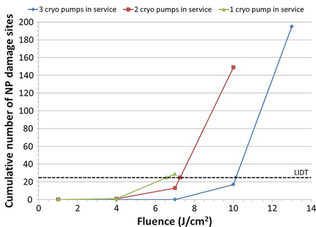
Fig. 6 Cumulative number of NP damage sites in the AR coatings for normal incidence at 532 nm.
