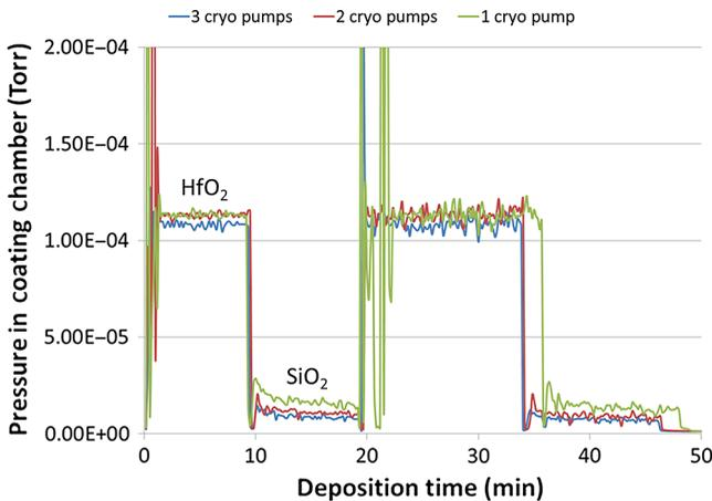
**Fig. 3** Total pressure in the coating chamber during the deposition of the AR coatings.
