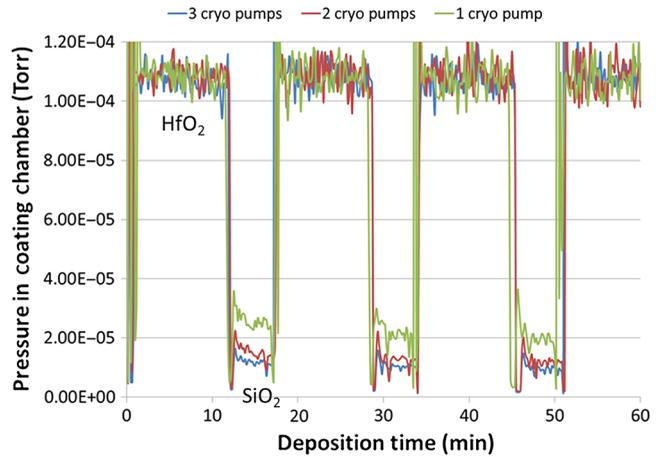
**Fig. 4** Total pressure in the coating chamber during the deposition of the HR coatings. This figure captures the first seven layers of the deposition.
