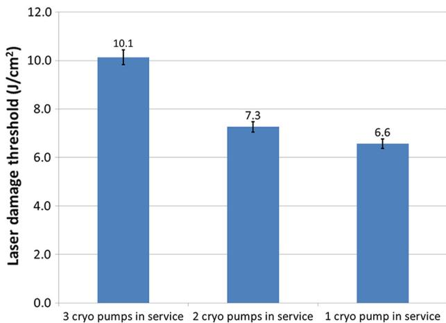
Fig. 5 LIDT data of the AR coatings at 532 nm and normal incidence.
