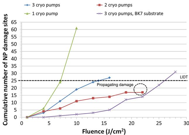
Fig. 8 Cumulative number of NP damage sites in the HR coatings at 532 nm, 45-deg AOI, P-pol.
