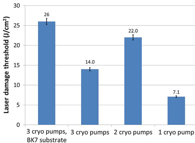
Fig. 7 LIDT data of the HR coatings at 532 nm, 45-deg AOI, P-pol.
