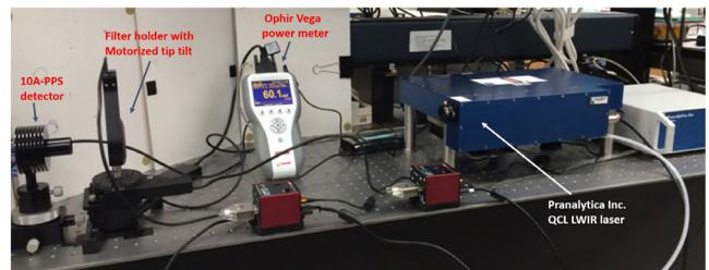
**Fig. 7** Experimental setup consisting of QCL tunable LWIR laser, Ophir–Spiricon pyrocam detector, rotating stage to hold filter sample and custom Labview interface for automated filter characterization.
