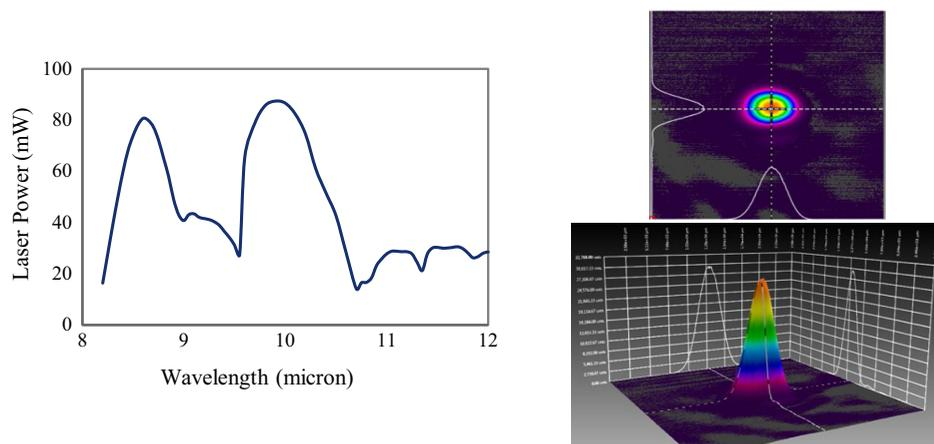
**Fig. 8** Measured laser power and a typical beam profile of a QCL.
