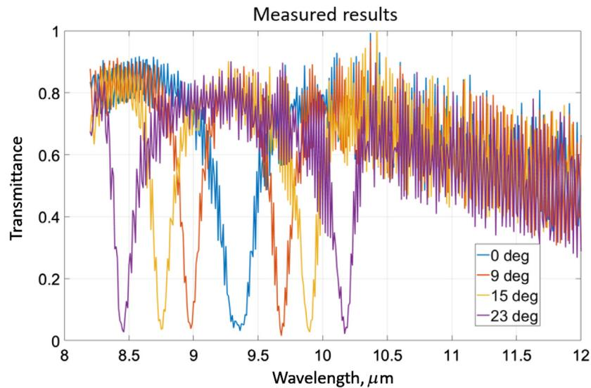
**Fig. 9** Measured 1-D GMRF transmission spectra for TE-polarized light at four incidence angles: 0 deg, 9 deg, 15 deg, and 23 deg.
