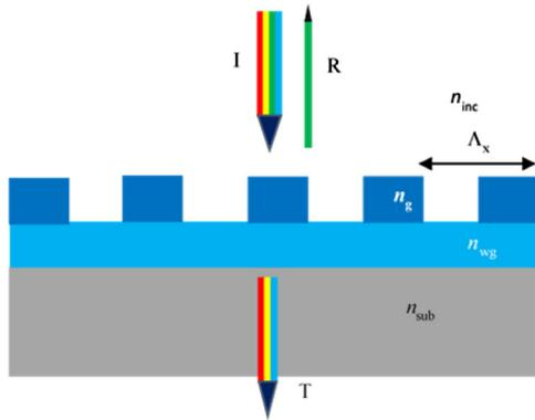
**Fig. 2** GMR grating-waveguide layers on a substrate schematically showing reflection at resonant wavelength and transmission at all other wavelengths due to coupling of one diffracted order in waveguide to excite leaky guided mode.
