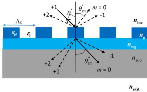
**Fig. 1** GMR grating-waveguide layers with diffractive orders illustrated;  $\epsilon_H$  and  $\epsilon_L$  represent dielectric permittivities for grating and no-grating regions. The refractive indices for each region are labeled.
