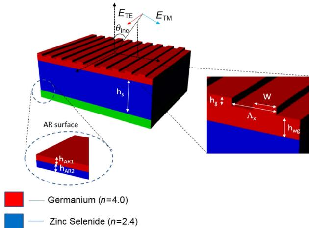
**Fig. 3** Basic GMRF configuration for a 1-D device. A grating and a planar waveguide are formed using Ge layers, which are deposited on top of a thick ZnSe substrate. An AR coating, composed of alternating layers of Ge and ZnSe, is deposited on the bottom surface of the substrate.  $W$  is the width of grating groove. The direction of incident light and polarization components are also shown.
