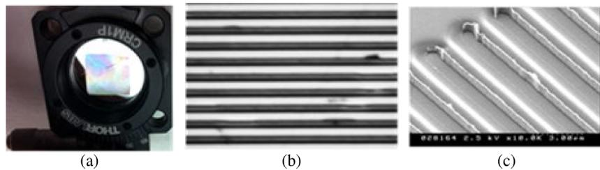
**Fig. 6** (a–c) Photo of 13- x 13-mm<sup>2</sup> filter, optical microscope picture of a fabricated device, and an SEM image.
