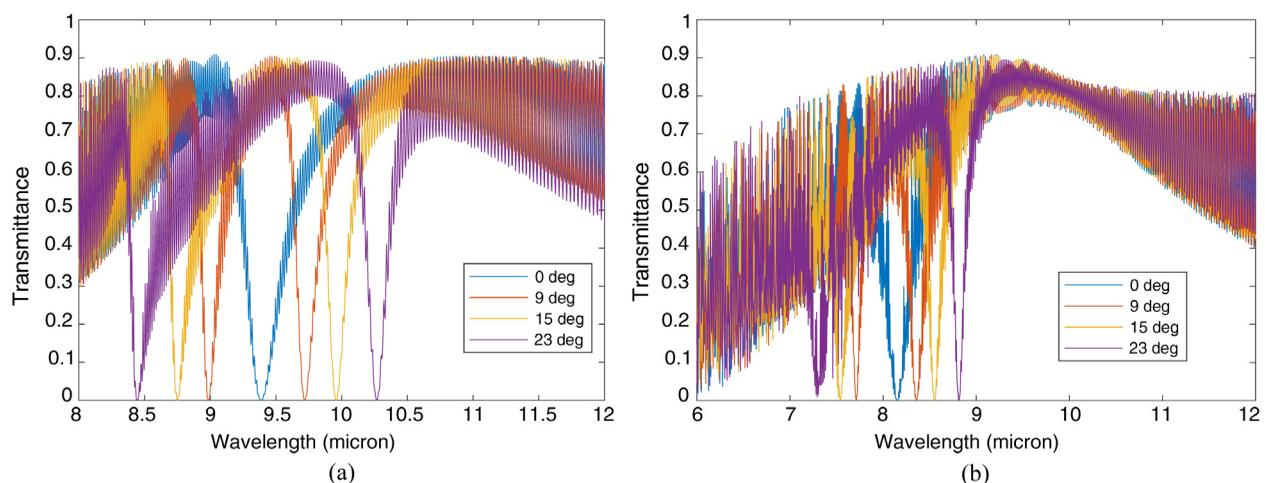
**Fig. 4** Simulated spectral transmittance plots using the RCWA method for the device parameters listed in Table 1. (a) Incident polarization is along the grating axis (i.e., TE) and (b) incident polarization is perpendicular to the grating axis (i.e., TM). The four curves are for incidence angles: 0 deg, 9 deg, 15 deg, and 23 deg.
