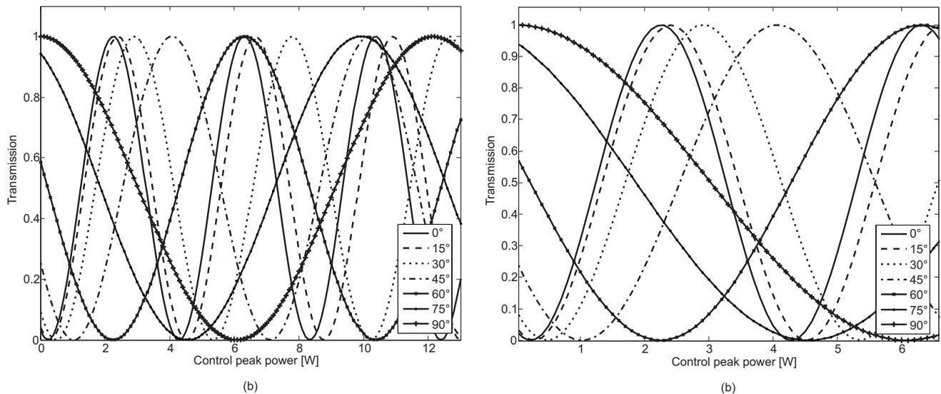
**Fig. 4** (a) Transmission of the NOLM, including the rotator versus the peak control-beam power and the mutual angles of polarization between the linearly polarized input data and control beam. (b) Zooms in on a part of Fig. 4(a).
