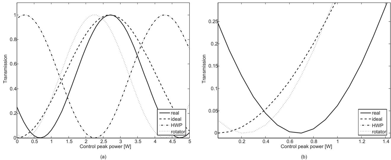
**Fig. 3** (a) Transmission of the NOLM as a function of the control-beam peak power for four different simulation schemes. HWP—a half-wave plate. (b) Zooms in on a part of Fig. 3(a).
