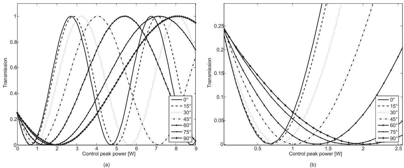
Fig. 2 (a) Transmission of the NOLM versus the peak control-beam power and the mutual angles of polarization between the linearly polarized input CW data and control beam. (b) Zooms in on a part of Fig. 2(a).
