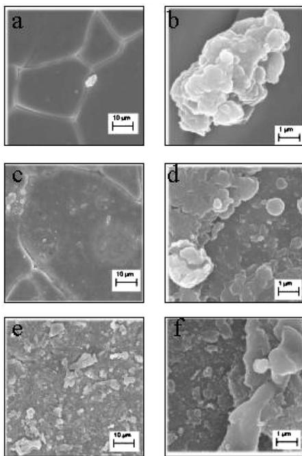
**Fig. 4** SEM images of PDLA deposits at different magnifications: (a) and (b) PDLA1, (c) and (d) PDLA4, (e) and (f) PDLA5.
