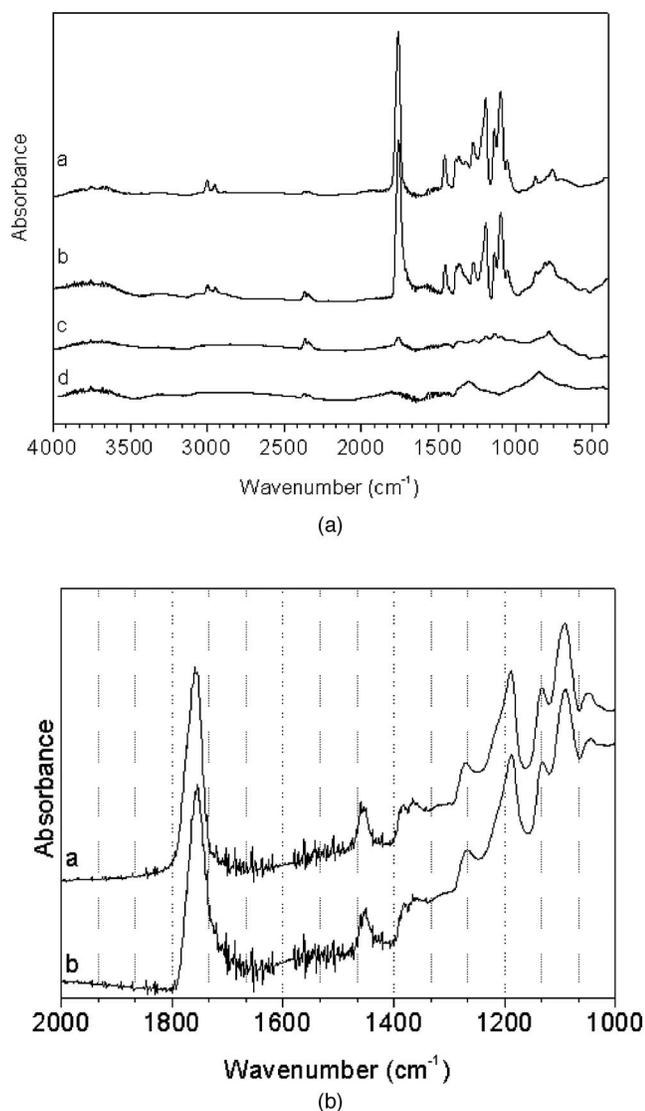
**Fig. 3** (a) FTIR spectra between 4000 and 400  $\text{cm}^{-1}$  of drop cast PDLLA (trace a), PDLLA5 (trace b), PDLLA4 (trace c), and PDLLA1 (trace d). (b) FTIR spectra of drop cast PDLLA (trace a) and PDLLA5 (trace b) between 2000 and 1000  $\text{cm}^{-1}$ .
