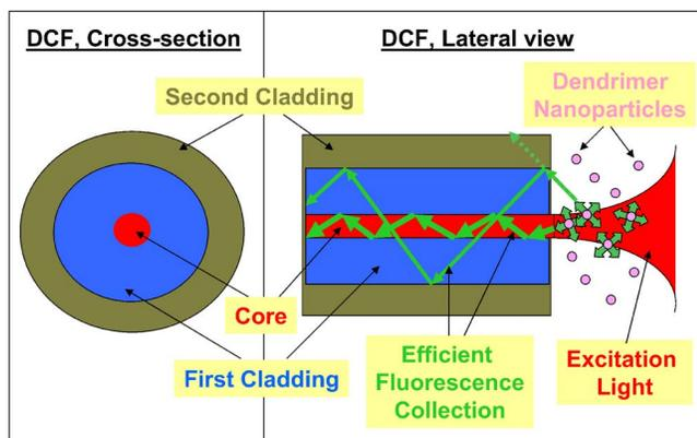
**Fig. 2** Schematic drawing of the DCF having a 10- $\mu\text{m}$  inner core, 123- $\mu\text{m}$  first cladding, and 178- $\mu\text{m}$  second cladding diameters. Unlike the SMF we have described previously, this newly developed DCF allows collection of emission fluorescence not only through the fiber core, but also through the inner cladding, resulting in increased efficiency.
