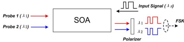
Fig. 1 Schematic diagram of the wavelength converter.
