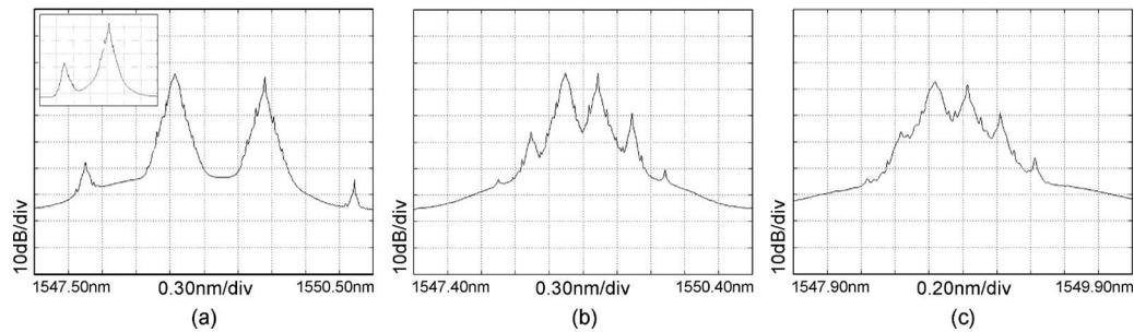
**Fig. 5** Optical spectrum of the obtained FSK signal with tone spacing of (a) 0.8 nm, (b) 0.3 nm, and (c) 0.2 nm. Inset: The optical spectrum of demodulated FSK.
