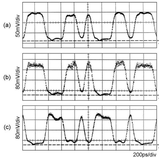
Fig. 3 Measured wave forms for (a) input signal, (b) converted signal at 1548.75 nm, and (c) converted signal at 1549.55 nm.
