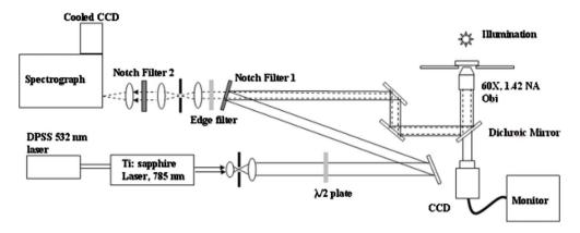
Fig. 1 Experimental setup. The solid line shows the trapping/excitation beam, whereas the dotted line indicates the Raman signal.
