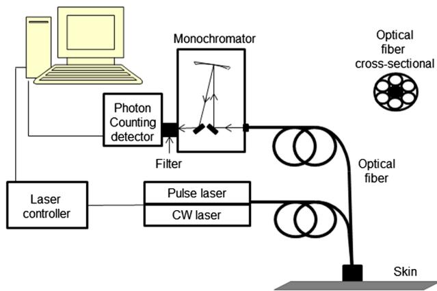
**Fig. 1** Experimental setup for skin autofluorescence lifetime measurements.
