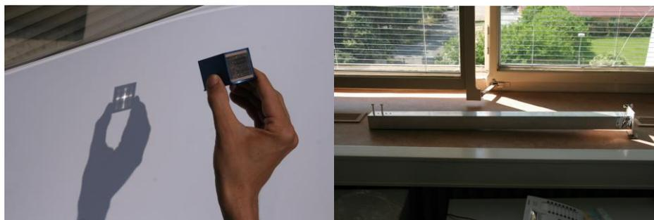
**Fig. 2** Imaging properties of the Mini 2D LE system – imaging of the Sun in optical light and The Mini 2D LE module with focal length of 900 mm (right).
