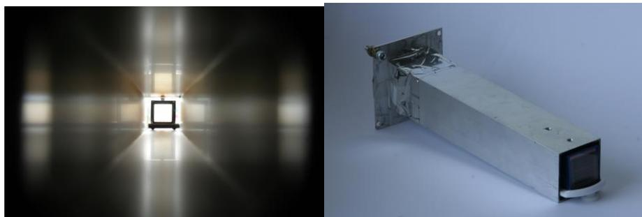
**Fig. 1** The Mini 2D LE objective with focal length of 250 mm suitable for application in cube and picosatellites. The inside view of the Mini 2D LE module (right).
