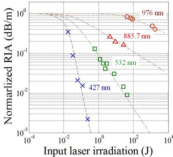
Fig. 2 the annealing efficiencies of the PA sources with different wavelengths.
