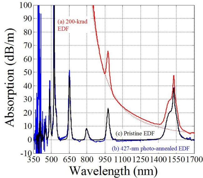
**Fig. 3** RIA spectra of (a) 200-krad  $\gamma$ -irradiated EDF, (b) 427-nm photo-annealed EDF, and (c) the pristine EDF.
