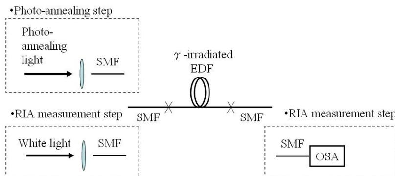
Fig.1. Schematic diagram of experimental setup for measuring photo-annealing induced RIA decreases.
