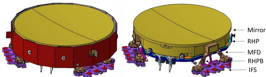
Fig 2: FCI M1 Mirror Assembly (MLI hidden on the right picture)
