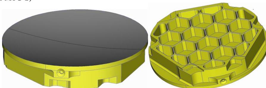
**Fig 3.3:** sketch of the M3 mirror for MTG-I (similar for MTG-S)
