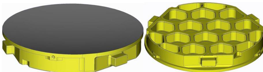
**Fig 3.1:** sketch of the M1 mirror for MTG-I (similar for MTG-S)
