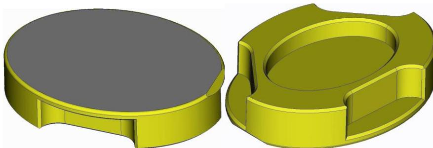
Fig 3.4.a: sketch of the M4 mirror for MTG-I
