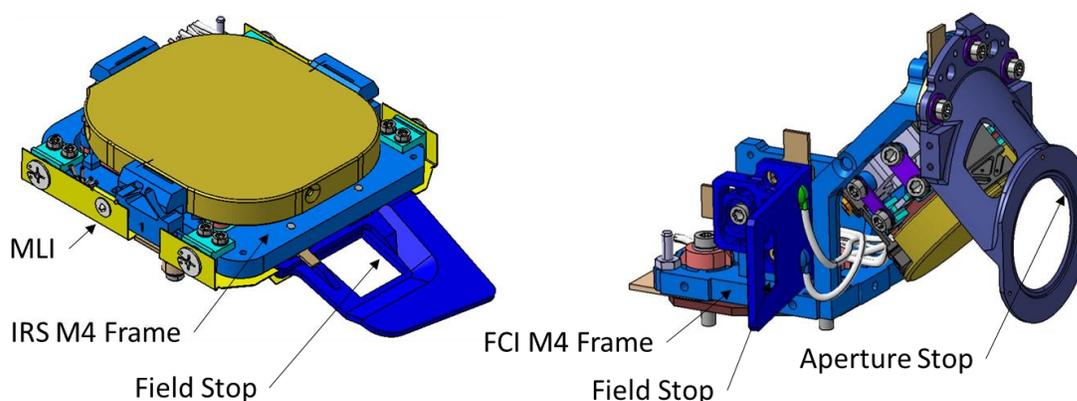
**Fig 4:** IRS M4 and FCI M4 Mirror Assemblies
