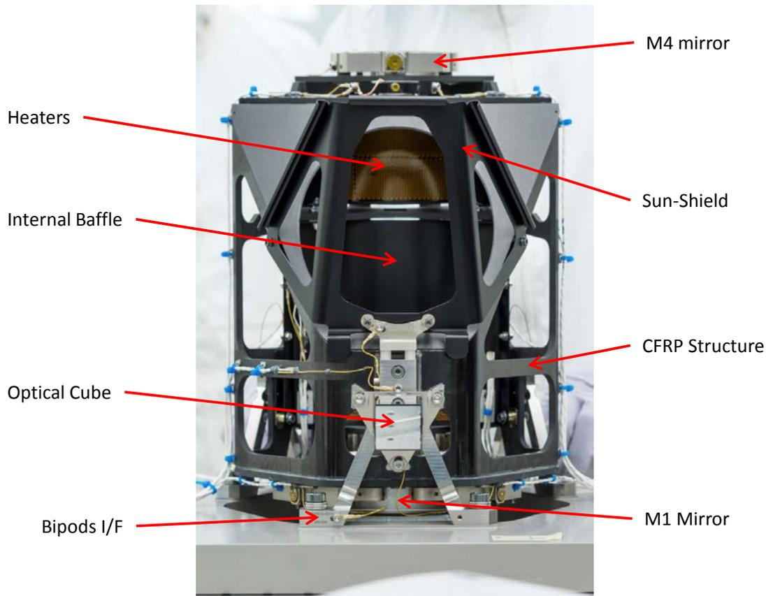
**Fig. 1. CaSSIS Telescope Assembly**
