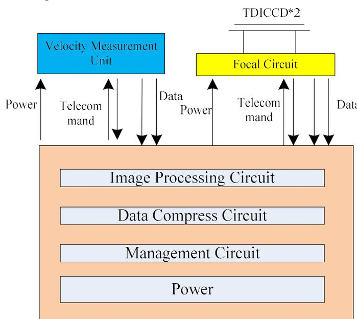
Fig. 9. The sketch of Integrated Circuits
