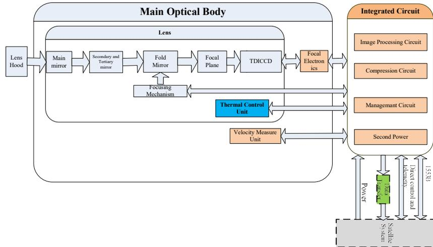
Fig. 5. The sketch of Hyper Resolution Camera
