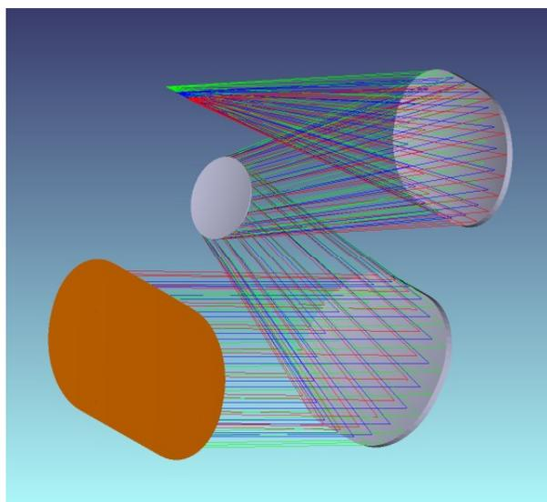
**Fig. 1.** Lay-out of the TMA.
