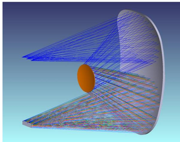
Fig. 3. Scheme of the Offner-type spectrometer.
