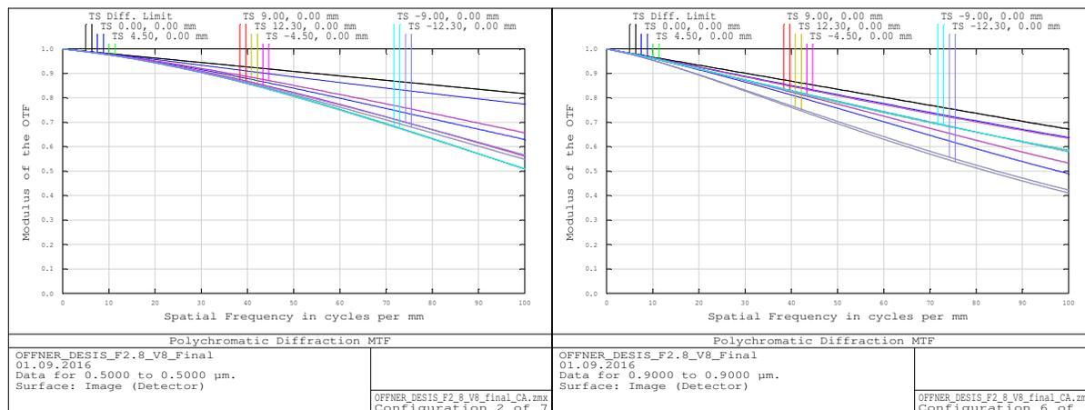
**Fig. 7.** Modulation transfer function (MTF) of the spectrometer for wavelengths of 500 nm (left), and 900 nm (right), respectively.
