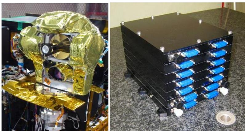
Fig 2. The optical (left) and electrical (right) part of the SOTA mounted on the SOCRATES
