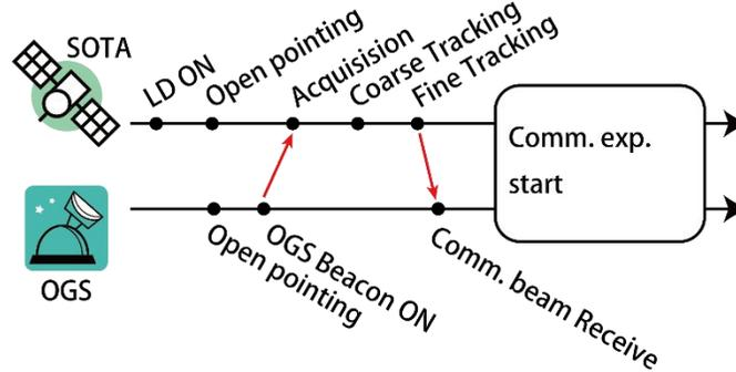
**Fig. 5.** Sequence of events for optical communication experiment
