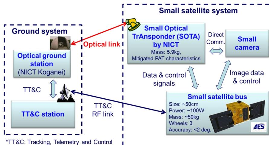
**Fig. 1.** Configuration of Space Optical Communications Research Advanced Technology Satellite (SOCRATES).
