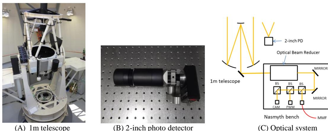
**Fig. 3.** Optical ground station and optical system
