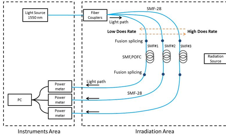
Fig.1 Schematic diagram of coil's RIA measurement setup
