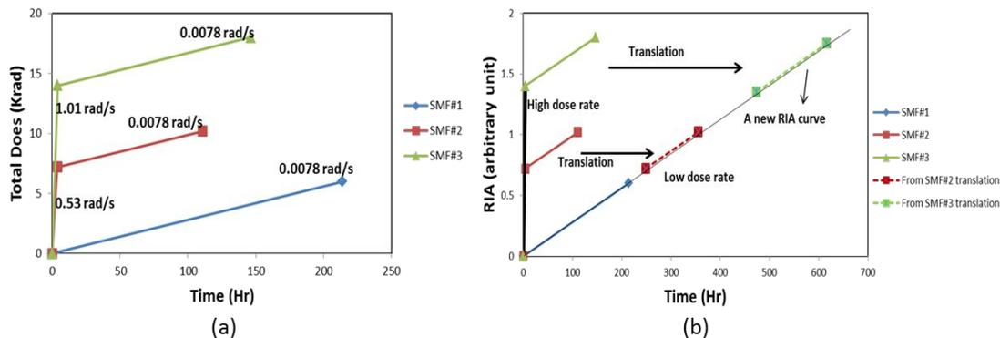
Fig.2. (a) The irradiation treatments of total dosages and dose-rates for the three coils. (b) Acquiring a new RIA curve with low dose-rate by the switching dose-rate method
