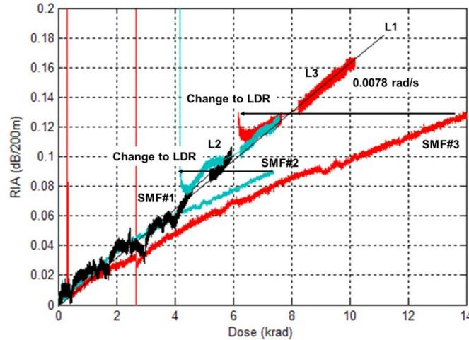
Fig.3. The result of an accelerated gamma irradiation test of low dose-rate (LDR) for SMF
