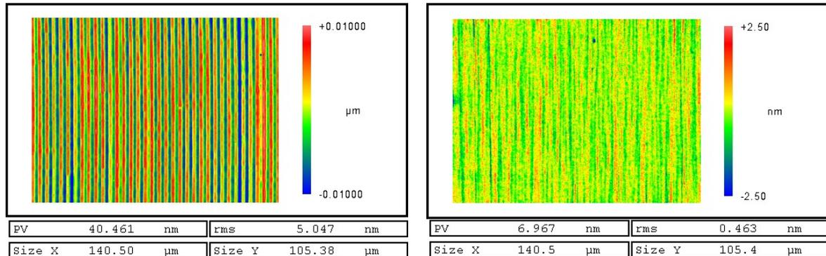
**Fig. 1.** Roughness of a metal mirror (magnification 50x; measuring range 141μm x 105μm); left: after diamond turning with typical pattern; right: after MRF polishing [8].
