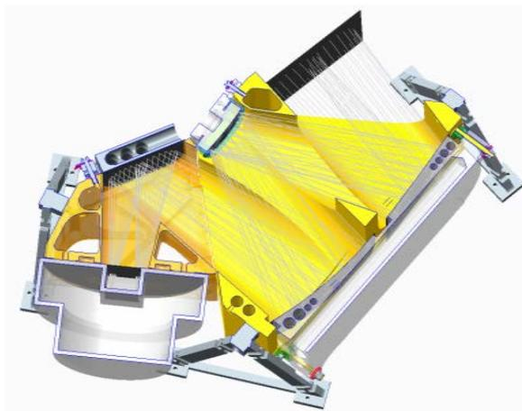
**Fig. 9.** CAD model of the complete TMA including FPA dummy at the left hand side, the bipods (left and right hand side of the M1-M3 substrate between FPA dummy and M2 mirror), ray bundles, and mirror intersection.
