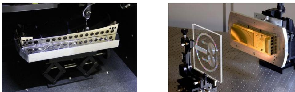
**Fig. 6.** Measurement of the mirror module in the profilometer UA3P 650H from Panasonic with a  $5 \mu\text{m}$  diamond stylus at Fraunhofer IOF (left); measurement setup with multi aperture CGH for a smaller mirror module, sample from PREMIER instrument (right) [5; 8; 10; 13].
