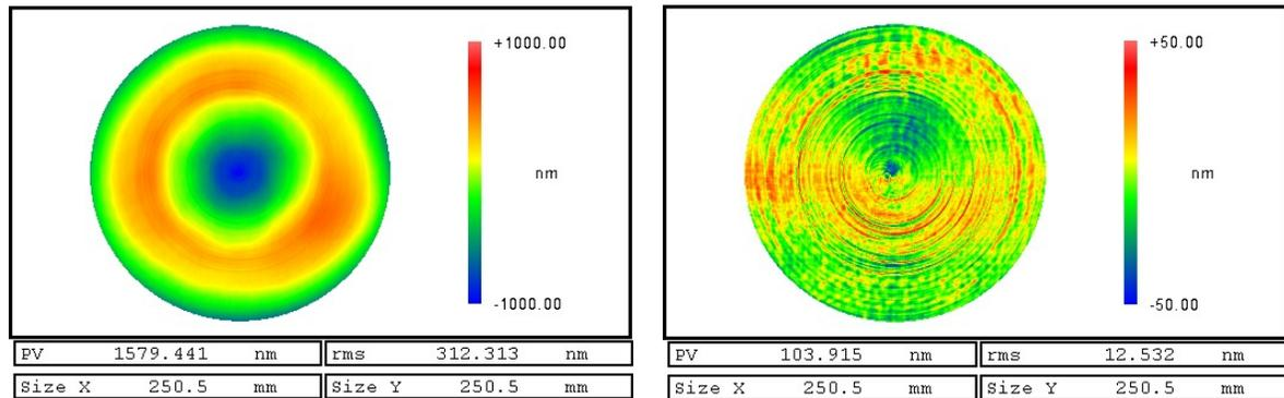
**Fig. 2.** Shape deviation of curved metal optics (diameter: 250 mm; freeform mirror with approx. 400 μm unsymmetry); left: after slow-tool diamond turning; right: after MRF polishing (three cycles).
