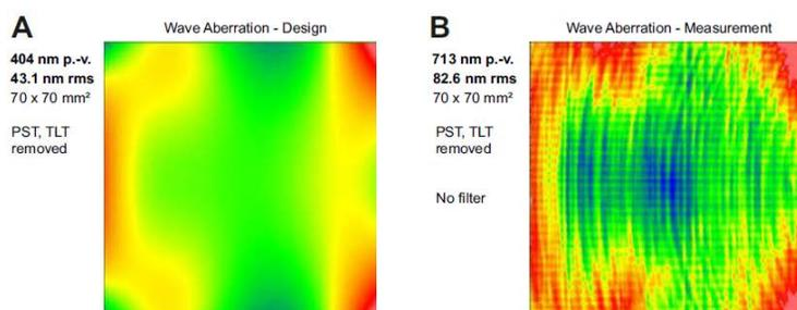
**Fig. 11.** Experimentally determined system wavefront of the anamorphic telescope in the central field point, A: designed wavefront 404 nm p.-v. / 43 nm rms; B: measured wavefront 713 nm p.-v. / 83 nm rms [14].
