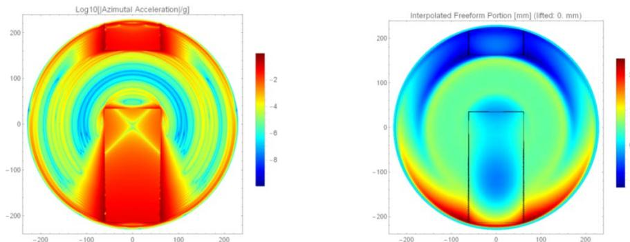
**Fig. 4.** Manufacturing analysis; left: azimuthal acceleration of the tool; right: freeform portion (equivalent to fast tool travel) for diamond turning of both optical surfaces in a single tool path for mirror module M1-M3.
