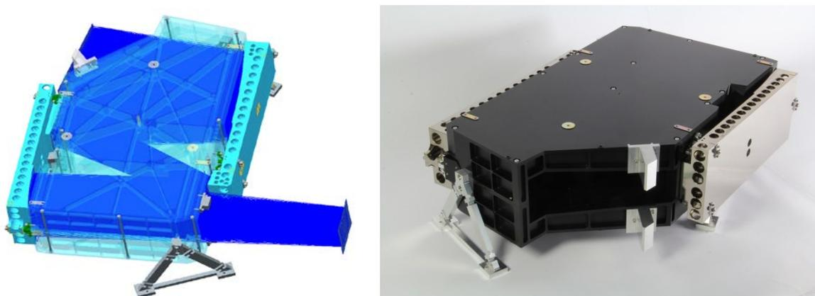
**Fig. 10.** CAD model of the complete telescope (left); final telescope demonstrator (right) [14].
