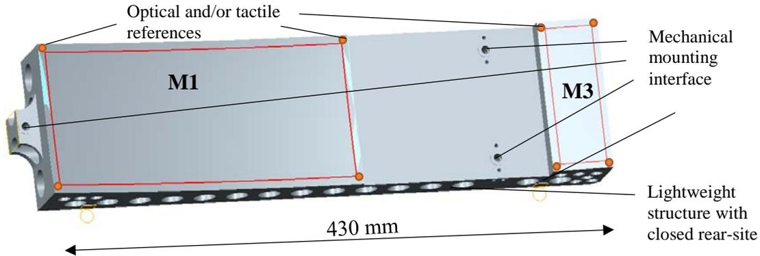
**Fig. 3.** CAD layout of the mirror module M1-M3 including the optical surfaces M1 and M3, ultra-precisely machined mounting interfaces, and reference spheres for tactile and/or interferometric metrology.
