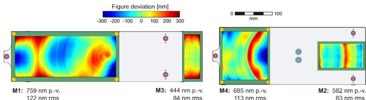
**Fig. 7.** Shape- and relative position deviations of the mirror modules M1-M3 (left) and M2-M4 (right) after ultra-precise diamond machining [14].
