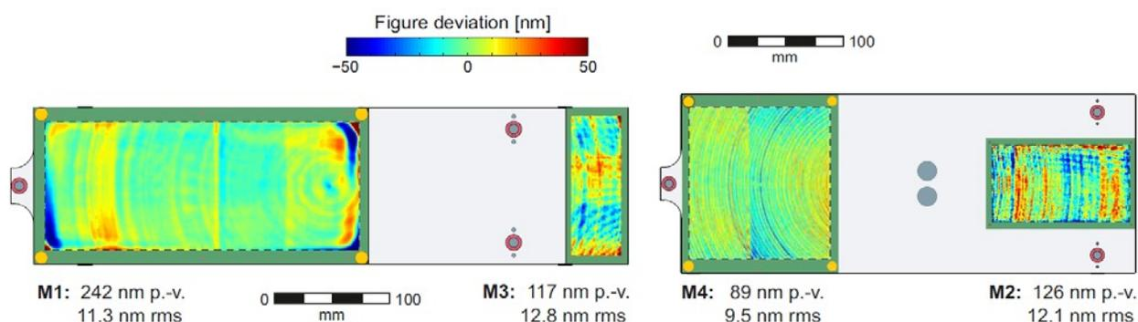
**Fig. 8.** Shape- and relative position deviations of the mirror modules M1-M3 and M2-M4 after MRF [14].
