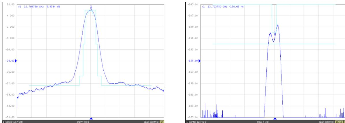
**Fig. 4.** Photonic RF filter response for 36 MHz bandwidth and corresponding mask. (Left) Amplitude. (Right): Group delay.
