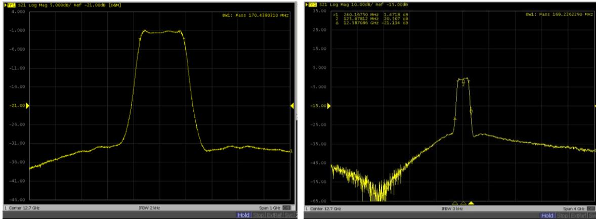
**Fig. 7.** Photonic RF filter response for 72 MHz bandwidth and corresponding mask. (Left) Amplitude. (Right): Group delay.
