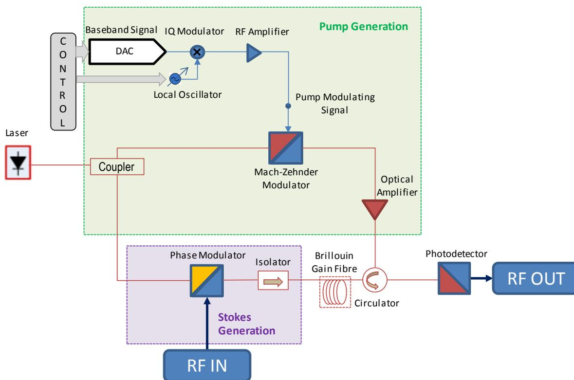
**Fig. 1.** Photonic RF filtering architecture
