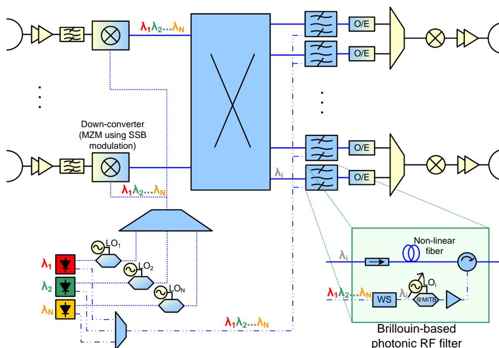
Fig. 8. Photonic payload architecture integrating Brillouin-based photonic RF filtering
