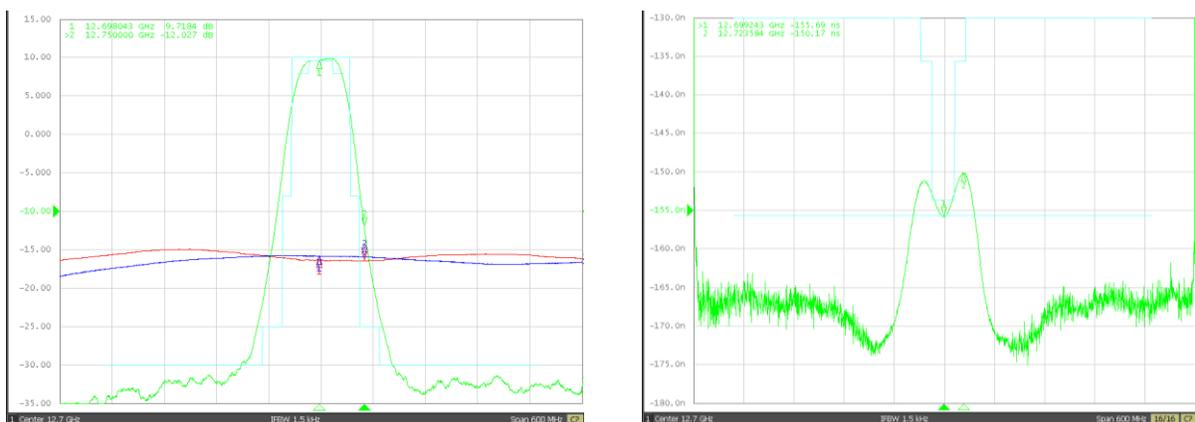
**Fig. 5.** Photonic RF filter response for 54 MHz bandwidth and corresponding mask. (Left) Amplitude. (Right): Group delay.
