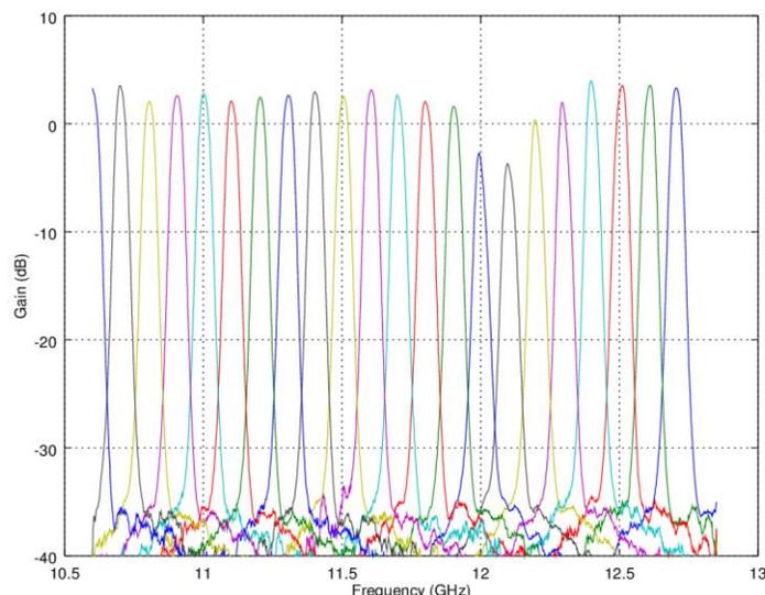
**Fig. 3.** Photonic RF filter gain response tuning within the entire Ku-band
