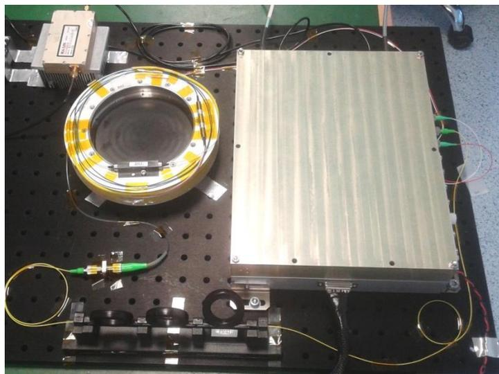
**Fig. 2.** Photonic RF filtering demonstrator
