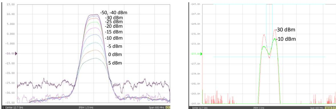
**Fig. 8.** Photonic RF filter response as a function of RF input power. (Left) Gain. (Right) Group delay
