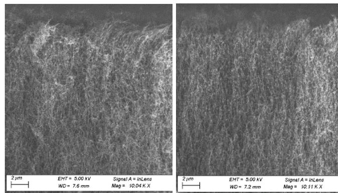
**Fig. 7.** SEM cross section of the top surface of VACNTs (sample G) before and after O<sub>2</sub> plasma etch.
