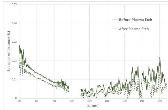
**Fig. 6.** Specular reflection spectra of VACNTs (sample G) before and after O<sub>2</sub> plasma etch.
