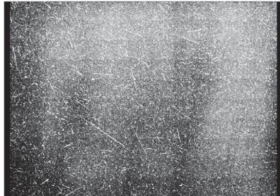
Fig. 7. Dark signal measurement with exposure time 136 seconds and gain factor 40 in South Atlantic Anomaly (SAA). The increased number of random hits and trails of particles can be observed.
