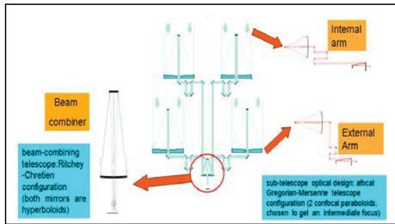
Fig. 1: interferometer optical design
