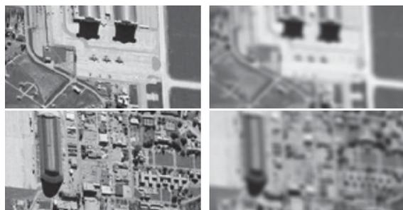
Fig. 3- Original (left) and space variant blurred (right) test images. Top – low spatial frequency content. Bottom – high spatial frequency content
