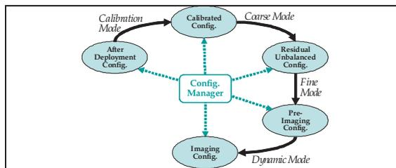
Fig. 6. Configurations and Modes of Alignment.
