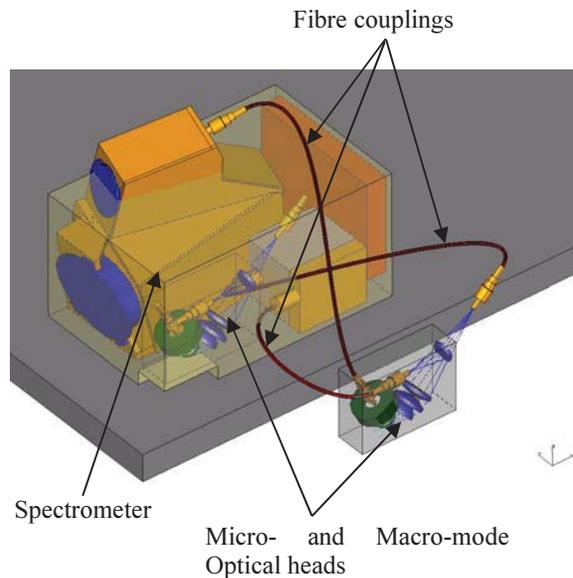
Fig. 6. EBB mechanical layout [8].
