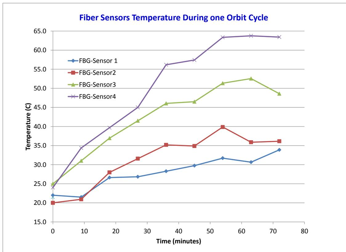
Fig. 6: Temperature measurements provided by the four sensors of Fiber Line\_sens6(Bus)
