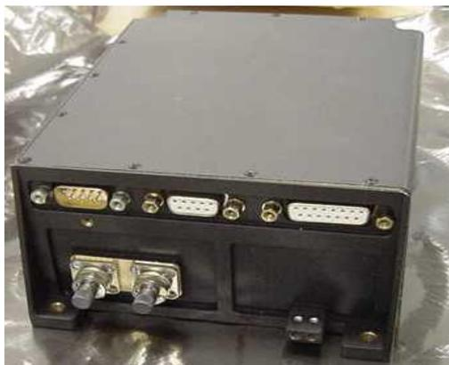
**Fig. 3: Photograph of the Interrogation module**
