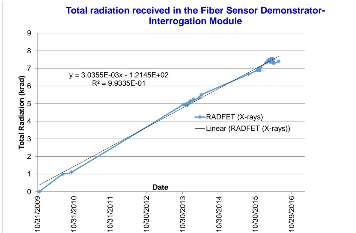
Fig. 9: Calibration of the RADFET vs the time spent in space
