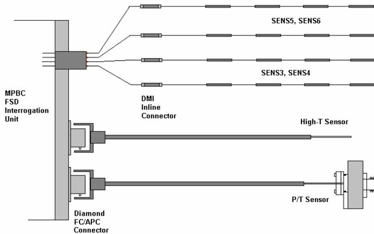
**Fig.1 Schematic of FSD fiber-optic sensor signal harness.**
