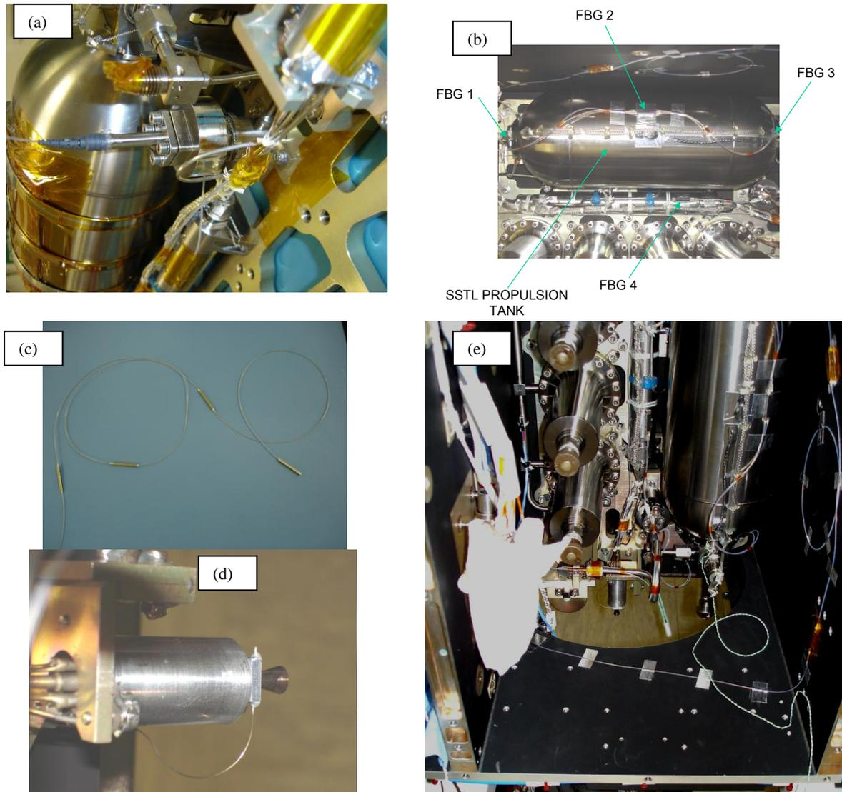
**Fig. 2: Photograph of flight P/T sensor integrated with the SSSL propulsion system for Proba-2**
