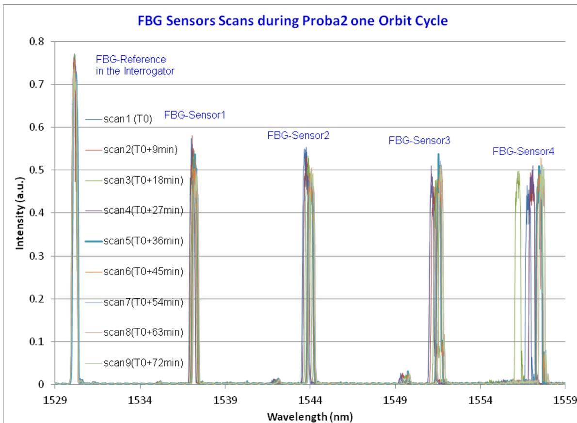
Fig. 5: Scan of the wavelengths of the Line during the orbit cycle
