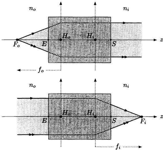
Figure 7. Focal points and focal lengths.
