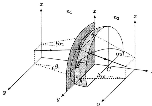
**Figure 2. Refraction at a spherical interface.** The ray travels through a spherical interface with extreme refractive index  $n_1$  and  $n_2$ . It hits the refractive surface in  $\underline{x}_1 = x + iy$  with an optical angle  $n_1\underline{\alpha}_1 = n_1(\alpha_1 + i\beta_1)$ , and leaves it from the same point  $\underline{x}_2 = x + iy$  with an optical angle  $n_2\underline{\alpha}_2 = n_2(\alpha_2 + i\beta_2)$ .
