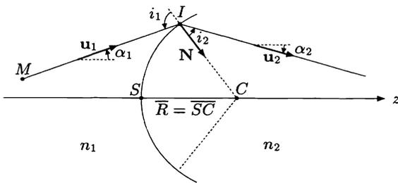
**Figure 10. Refraction at a spherical interface with sign conventions.**
