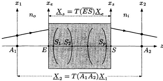
Figure 3. Propagation through an optical system.
