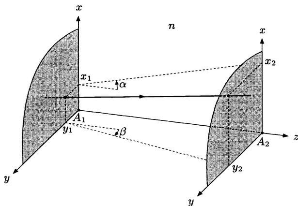
**Figure 1. Propagation through free space.** The ray travels in a homogeneous medium with constant refractive index  $n$ . It leaves the first front plane from  $\underline{x}_1 = x_1 + iy_1$  with an optical angle  $n\underline{\alpha}_1 = n(\alpha + i\beta)$ , and hits the second one with the same optical angle  $n\underline{\alpha}_2 = n(\alpha + i\beta)$  in  $\underline{x}_2 = x_2 + iy_2$ .
