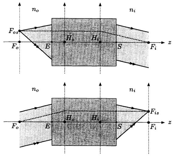
Figure 8. Focal planes and secondary focal points.
