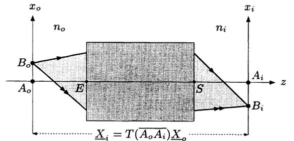
Figure 4. Transfer between two conjugate planes.
