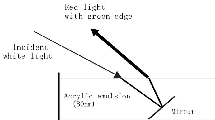
Figure 7. Schematic diagram of demonstration of green flash.
