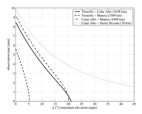
Figure 10. Maximum duration of simultaneous communication between ISS and two ground stations as a function of the elevation angle. (The distance cited in the insert is that between the stations.)
