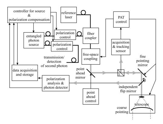
Figure 5. Block diagram of the transmitter terminal.
