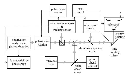
Figure 6. Block diagram of the receiver terminal.
