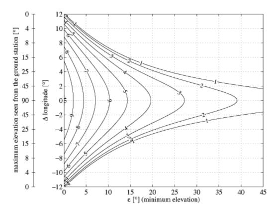
Figure 8. Maximum duration of communication between ISS and the OGS (given in minutes by the numbers inserted along the lines) as a function of the elevation angle and the difference in longitude of the ground station and the satellite when in zenith.
