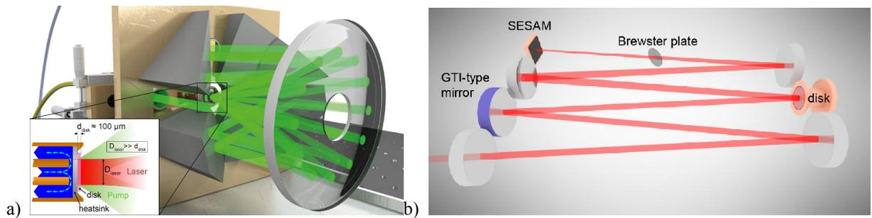
Figure 2 a) Illustration of thin-disk multi-pass pumping scheme b) Typical layout of SESAM modelocked thin-disk laser
