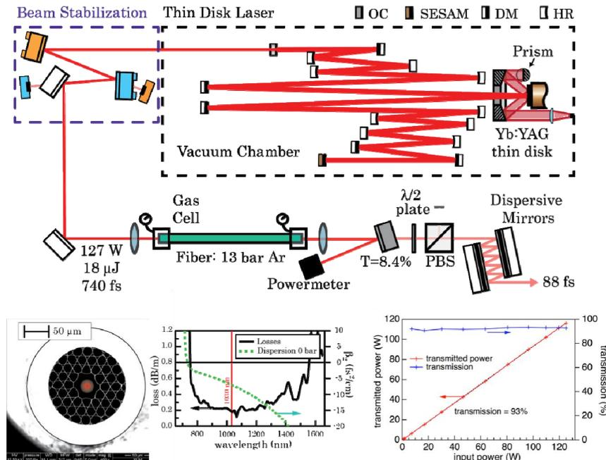
Figure 7 a) Experimental setup for the high average power pulse compression b) The low-loss 66 cm-long hypocycloid-core Kagome HC-PCF is hold in a gas chamber with 13 bar of Argon. The output is collimated and sent through a polarizing beam splitter (PBS) and a pair of dispersive mirrors c) The transmission through the fiber alone reaches up to 118 W of output average power (93% of transmitted power).
