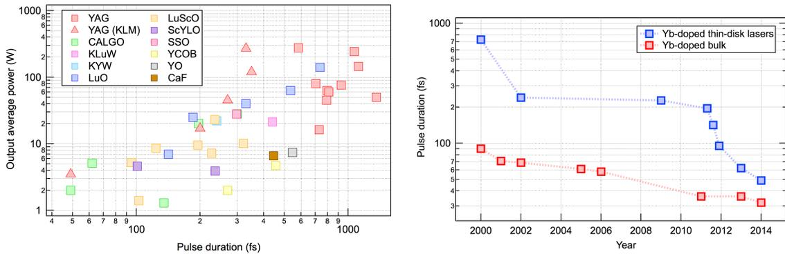
Figure 6 – a) Output average power of demonstrated modelocked TDLs based on different gain materials, showing the ongoing challenge of achieving short pulse durations and high average power levels b) Evolution of pulse duration available from modelocked thin disk lasers: reducing the pulse duration from state-of-the-art high-power systems represents one major milestone.
