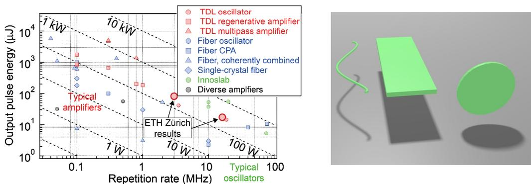
Figure 1. a) State-of-the-art of high-power ultrafast laser systems. Different technologies have been pushing the average power frontiers, recently surpassing the kilowatt milestone. b) illustration of different laser geometries suitable for high-power lasers (fibers, slabs, disks).
