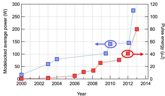
Figure 3. Evolution of average power and pulse energy of modelocked thin-disk oscillators since their first demonstration in the year 2000
