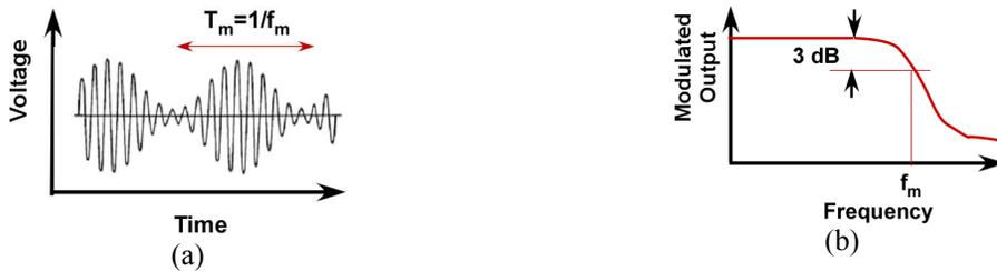
Figure 3. Modulated output (a) and the definition of the maximum modulation frequency  $f_m$  (b).
