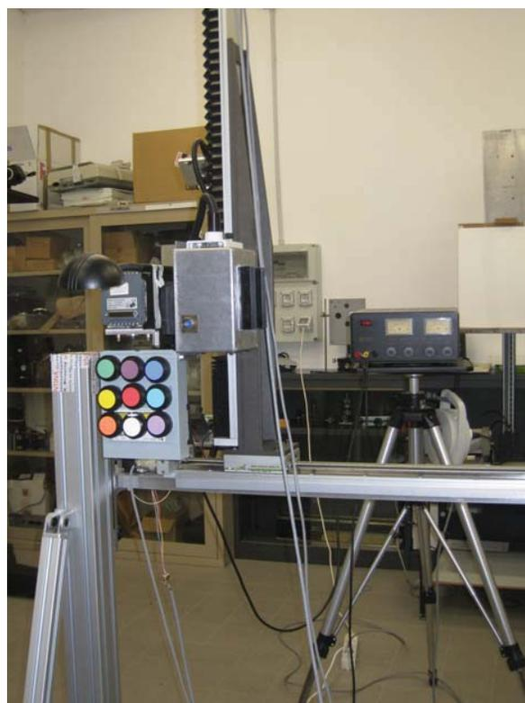
Figure 2. (a): Laboratory set up employed for testing imaging interferometer performances showing both ceramic tiles mounted on the sledge and the interferometer prototype (b): Colored ceramic tiles mounted on the motorized sledge (b).
