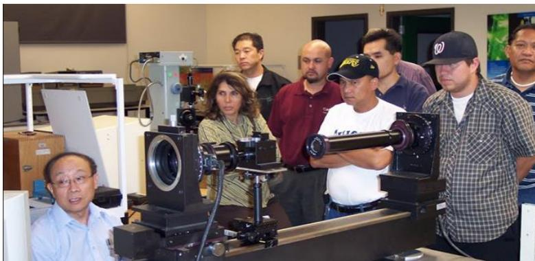
Fig. 5 is a photograph of IVC ATEP students in 2007. At this time the focus of the Laser Electro-optics Technology Program was more on optics. Here they are learning about optical performance testing using an MTF Bench.
