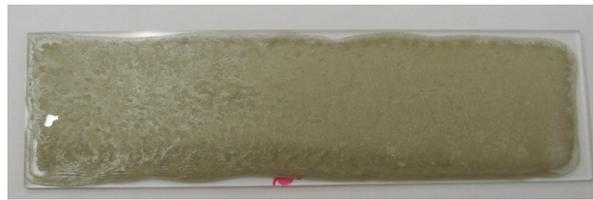
Figure 2. Ag + DNA-CTMA EMI shield sample.
