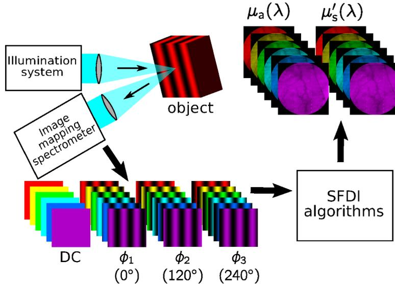
Figure 1: The experiments involve illuminating the sample with broadband light in a sequence of 4 different spatial patterns. The first pattern is unmodulated (DC), while the following three are each modulated by the same spatial frequency but are shifted in phase from one another by  $120^\circ$ . The remitted light is captured by the IMS imaging spectrometer, so that then SFDI algorithms produce two cubes of data:  $\mu_a(x, y, \lambda)$  and  $\mu'_s(x, y, \lambda)$ .
