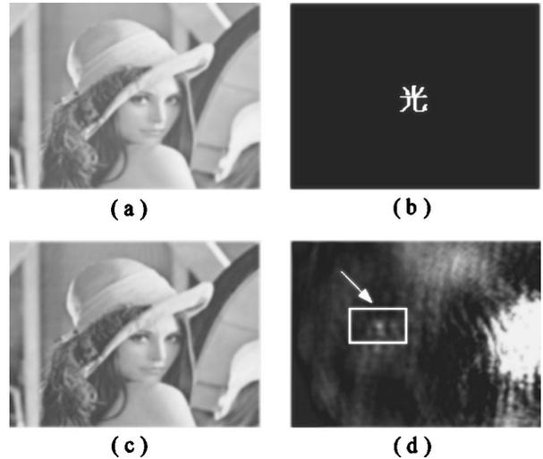
Fig. 3 Experimental results of correlation-based watermarking using constant-level embedding algorithm with weight value  $\alpha=0.2$ : (a) cover image, (b) mark pattern, (c) watermarked image (PSNR=25 dB), and (d) detected correlation.
