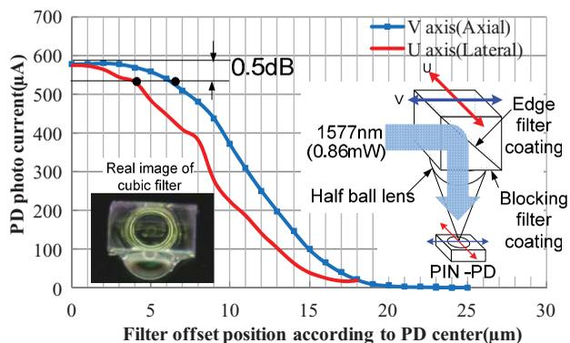
Fig. 3 Measured PD photocurrent output according to filter offset from the center of the PD.
