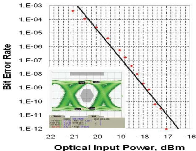
Fig. 4 Measurement results of the receiver's 10-Gbps sensitivity and eye diagram of limiting amp output at PRBS  $2^{31}-1$ ,  $10.3125$  Gbps.
