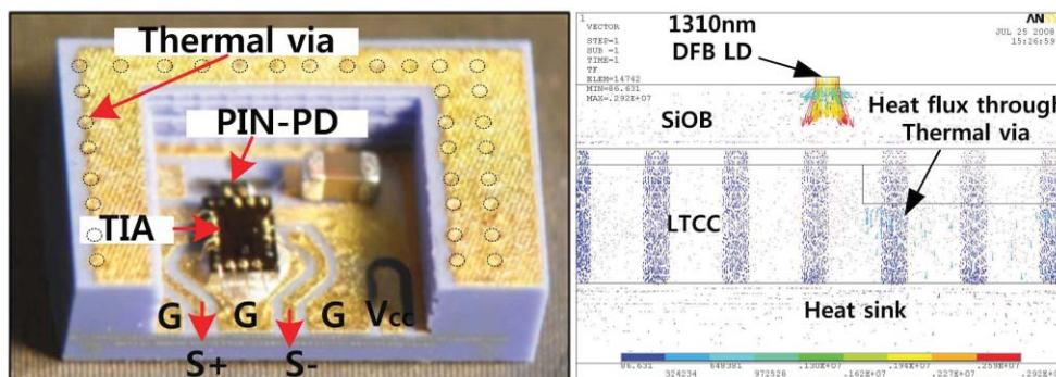
Fig. 2 High resistance LTCC substrate for noise sensitive 10-Gbps PIN-TIA receiver and heat flux vector through thermal via.
