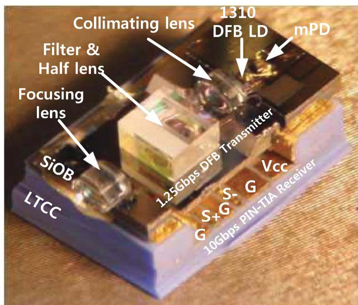
Fig. 1 Compact BOSA stacked transmitter and receiver for small footprint ( $4 \times 6 \times 2.5 \text{ mm}^3$ ).
