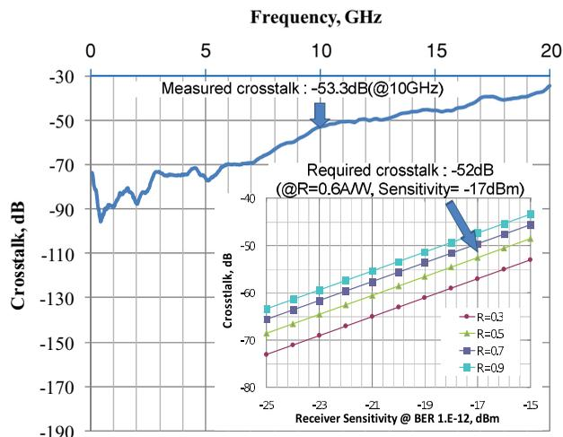
Fig. 5 Minimum required transmitter-receiver electrical cross talk for TIA and measurement results.
