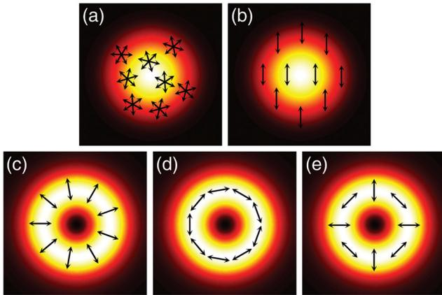
**Fig. 1** Polarization distribution of (a) natural, unpolarized light, (b) linearly polarized beam, (c) RPB, (d) APB, and (e) hybridly polarized beam.
