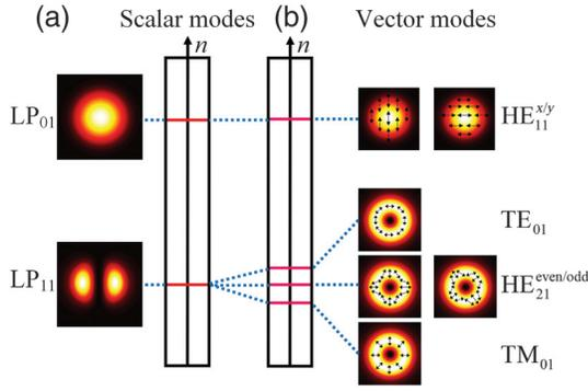
**Fig. 3** Mode distributions of TMF under (a) scalar approximation and (b) corresponding groups of the vector modes. Adapted with permission from Ref. 80 © OSA Publishing.
