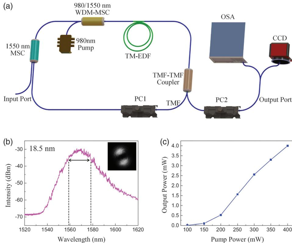
**Fig. 6** (a) Configuration of the all-TMF laser for  $LP_{11}$  mode oscillation. TM-EDF, two-mode erbium-doped fiber; PC, polarization controller; OSA, optical spectrum analyzer; CCD, charge coupled device; MSC, mode-selective coupler; WDM, wavelength division multiplexer. (b) Spectrum of the TMF laser; the inset shows the near-field pattern of the generated  $LP_{11}$  mode. (c) The relationship between the pump and output powers. Adapted with permission from Ref. 101 © OSA Publishing.
