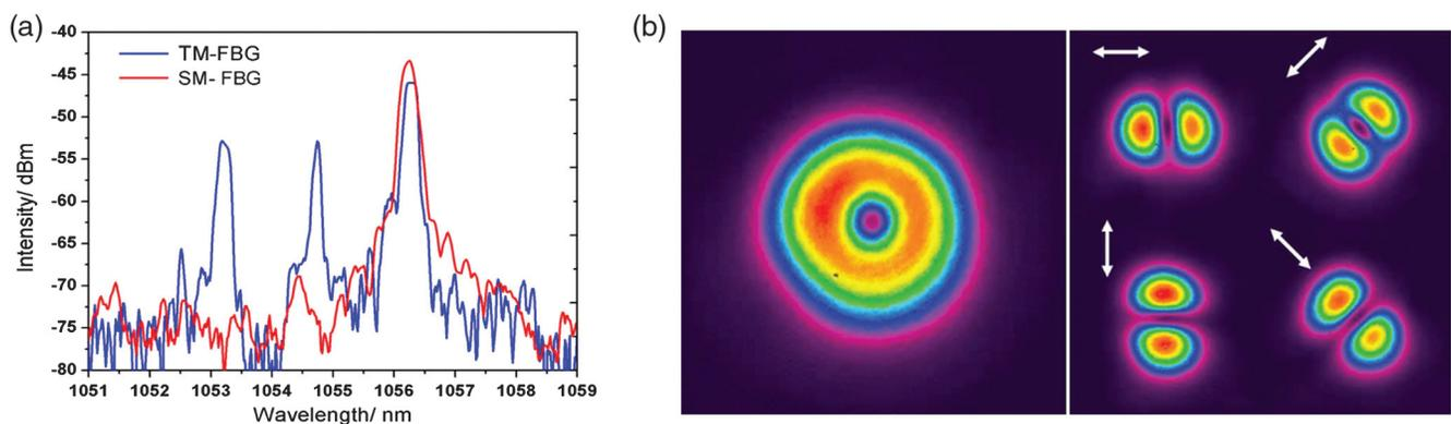
**Fig. 8** (a) Reflection spectrum of TMFBG and SMFBG. (b) Intensity distribution of radially polarized laser beam before and after passing through a linear polarizer with the transmission axis orientation denoted by arrows. Adapted with permission from Ref. 108 © OSA Publishing.
