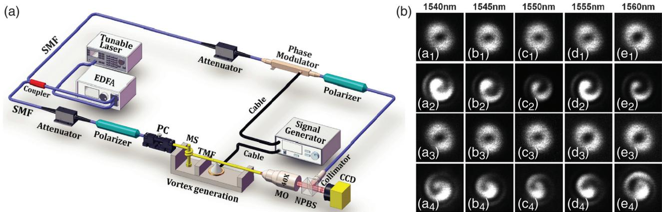
**Fig. 11** Generation of VBs based on an acoustically-induced LPFG. (a) Experiment setup. EDFA, erbium-doped fiber amplifier; SMF, single-mode fiber; PC, polarization controller; MS, mode stripper; TMF, two-mode fiber; MO, micro-objective; NPBS, nonpolarizing beam splitter; CCD, charge coupled device. (b) VBs and coaxial interference patterns at wavelengths of 1540, 1545, 1550, 1555, and 1560 nm. Adapted with permission from Ref. 118 © OSA Publishing.
