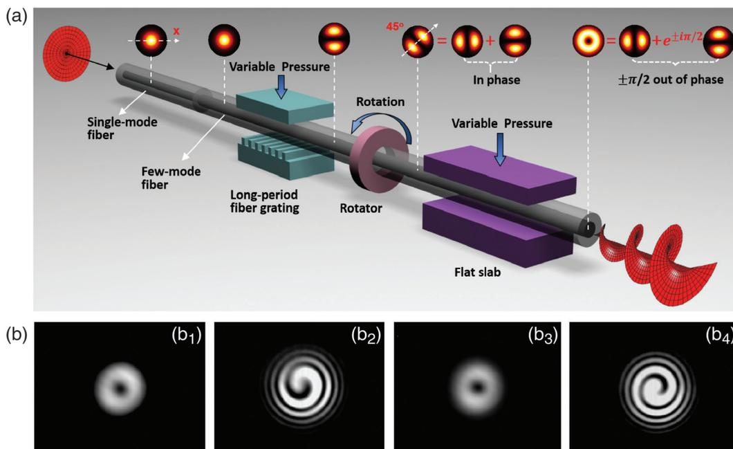
**Fig. 12** (a) Principle of the VB converter based on a mechanical LPFG. Intensity profiles of (b<sub>1</sub>) -1-order and (b<sub>3</sub>) +1-order VB. Coaxial interference patterns of (b<sub>2</sub>) -1-order and (b<sub>4</sub>) +1-order VB with a Gaussian beam. Adapted with permission from Ref. 120 © OSA Publishing.
