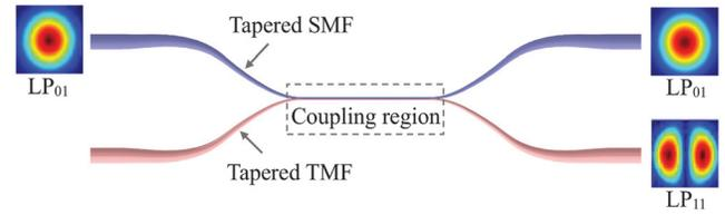
Fig. 5 Mode-selective coupler based on tapered SMF and TMF.
