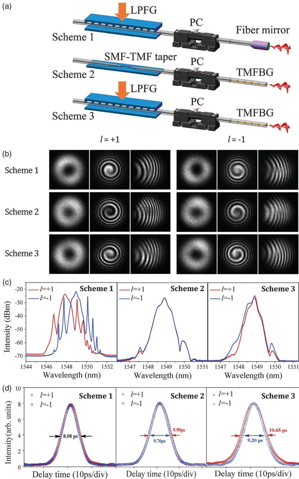
**Fig. 13** (a) Mode coupling and output elements are the LPFG and fiber mirror, SMF-TMF taper and TMFBG, and LPFG and TMFBG for schemes 1, 2, and 3, respectively. (b) Intensity distributions and interference patterns, (c) optical spectra, and (d) autocorrelation traces of mode-locked vortex lasers.  $l$ , topological charge. Adapted with permission from Ref. 130 © AIP Publishing.
