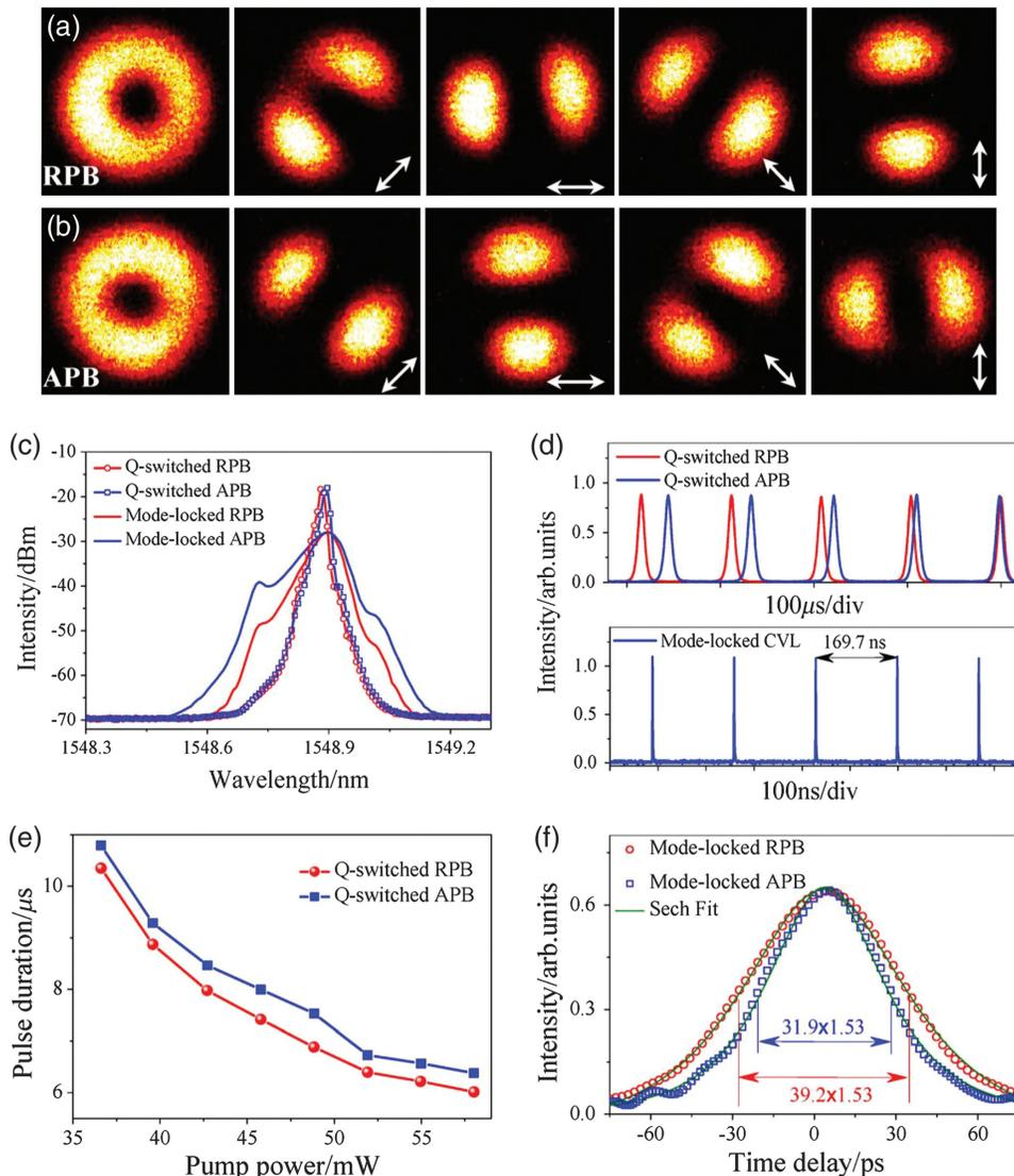
**Fig. 9** Q-switched and mode-locked cylindrical vector beam lasers. Mode-locked (a) RPB and (b) APB before and after passing through a polarizer. (c) Optical spectra and (d) pulse trains of Q-switched and mode-locked cylindrical vector beam lasers. (e) Evolution of Q-switched cylindrical vector beam lasers. (f) Autocorrelation traces of mode-locked cylindrical vector beam lasers. Adapted with permission from Ref. 105 © AIP Publishing.
