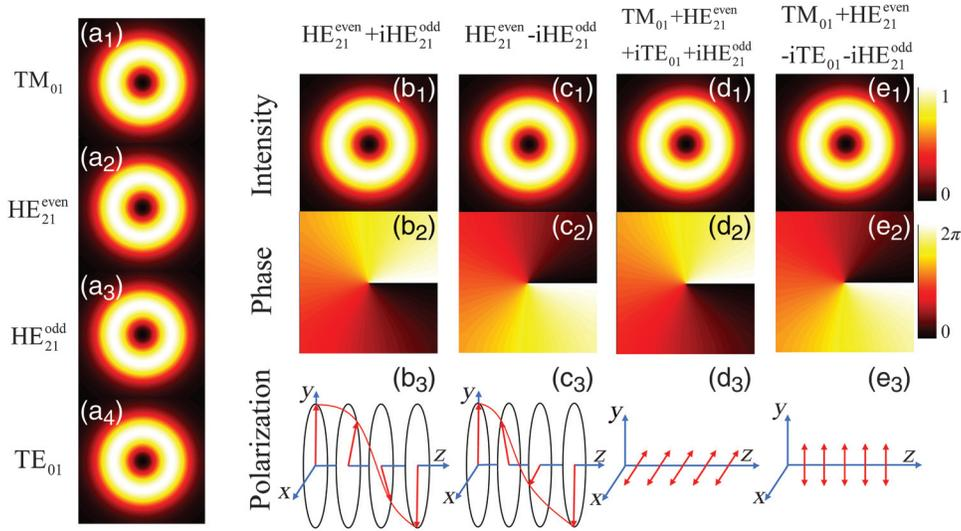
**Fig. 10** Formation mechanism of VBs in TMF. (a<sub>1</sub>)–(a<sub>4</sub>) mode distribution of TM<sub>01</sub>, HE<sub>21</sub><sup>even</sup>, HE<sub>21</sub><sup>odd</sup>, and TE<sub>01</sub> modes. Mode distribution, phase, and polarization of (b<sub>1</sub>)–(b<sub>3</sub>), (c<sub>1</sub>)–(c<sub>3</sub>) circularly polarized VBs and (d<sub>1</sub>)–(e<sub>3</sub>), (e<sub>1</sub>)–(e<sub>3</sub>) linearly polarized VBs.
