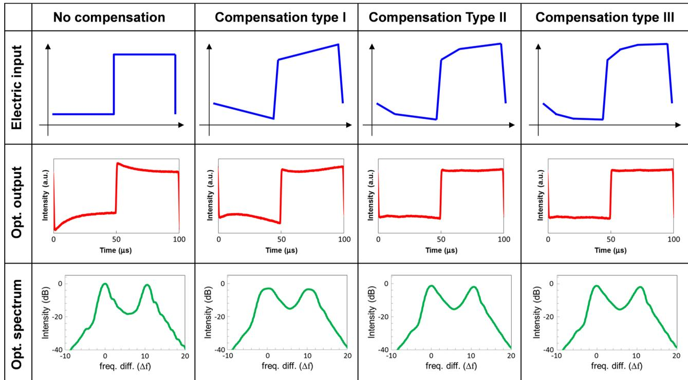
**Fig. 2** Four different types of electrical input waveforms (the first row) into a laser diode (LD) for generating two time-divided lightwaves and their optical output powers (the second row) and spectra (the third row).
