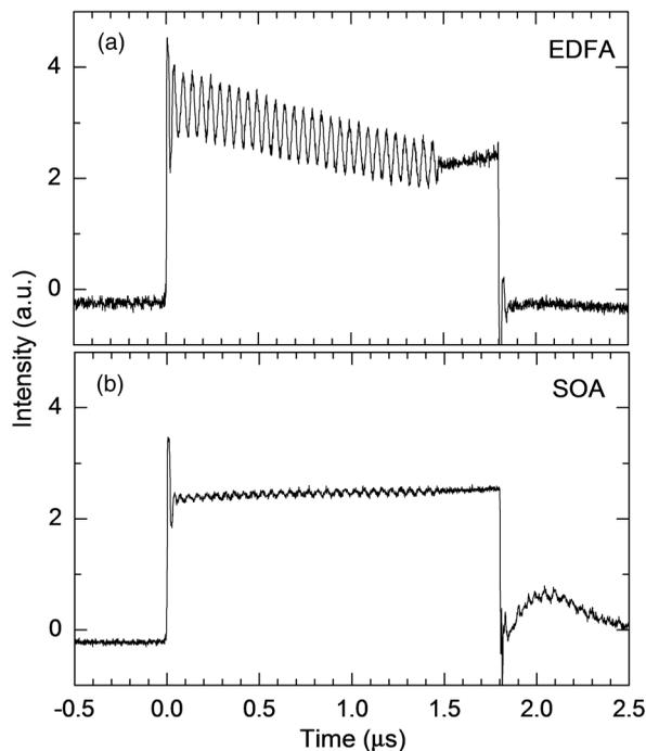
**Fig. 7** Amplified output power variations of a frequency-modulated pump lightwave after an erbium-doped fiber amplifier (a) and a semiconductor optical amplifier (b) according to time.
