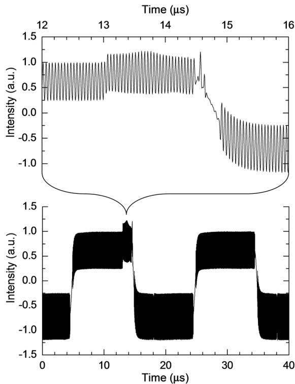
**Fig. 4** A power waveform of a probe lightwave measured after the stimulated Brillouin scattering amplification.
