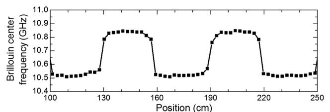
**Fig. 6** The center frequency shift in a Brillouin gain spectrum according to the optical fiber position.
