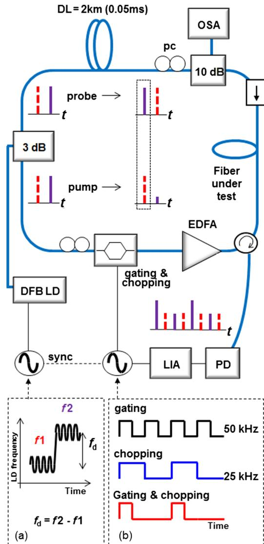
**Fig. 1** The schematic of the experiment setup with a modulated input function (a), and a gating and chopping function (b). A distributed feedback laser diode (DFB LD), lock-in-amplifier (LIA), and optical spectrum analyzer (OSA).
