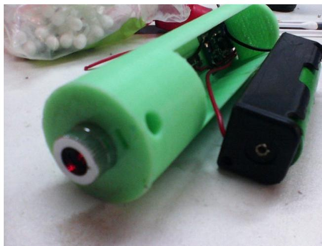
Fig. 5. The laser source mount
