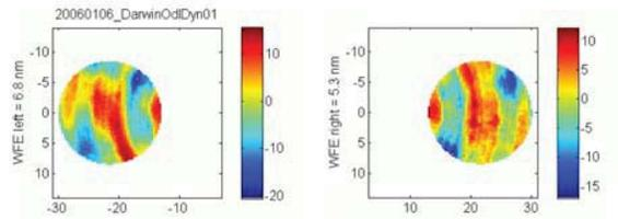
Fig. 9- Wave Front Error of Cat's Eye
