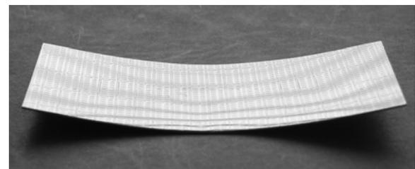
Fig. 12. Thermally formed (technology I) Si wafer to test cylinder (R = 150 mm, 72 x 23 x 0.625 mm).
