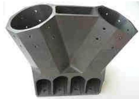
Figure III-8 view of the Si<sub>3</sub>N<sub>4</sub> end-fitting part
