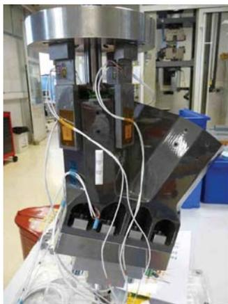
Figure IV-2 Proof test on the flight end fitting
