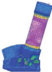
Figure III-10 FEM prediction of the test showing the stress distribution in the assembly (local highest stress peak is in end fitting when major large stressed area is in the beam)
