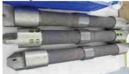
Figure III-5 Beams assembled by gluing and glued in Ta6V end fitting for tensile tests
