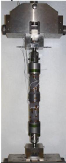
Figure III-6 Glued joined assembled beams for tensile test under tensile tests machine
