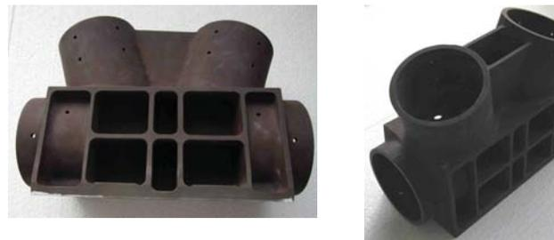
Figure III-13: Si3N4 demonstrator for the monolithic "truss bracket - M2 frame insert"
