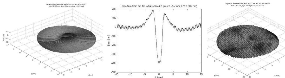
Fig. 9. Measurement of mid-spentials (spiral, centre defect and raster pattern from deterministic polishing)
