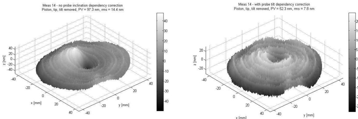
Fig. 6. Tilted flat measurement without (left) and with (right) the probe inclination dependency calibration
