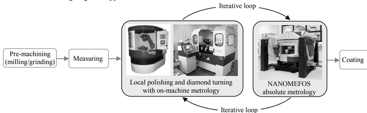
**Fig. 1.** Asphere and freeform production at TNO
