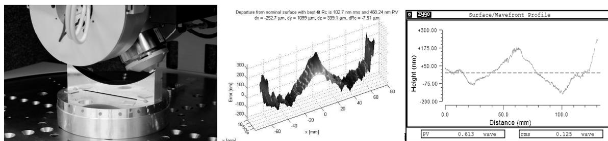
Fig. 8. Diamond turned freeform strip mirror (1 mm off-axis sphere), and NANOMEFOS and Zygo result
