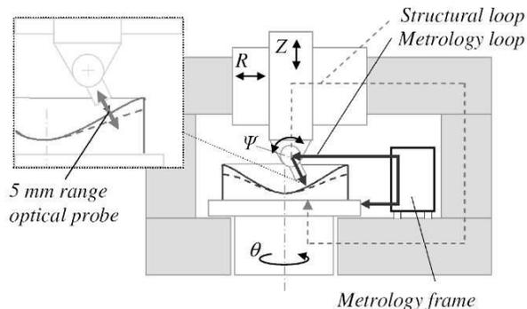
Fig. 2. Machine concept
