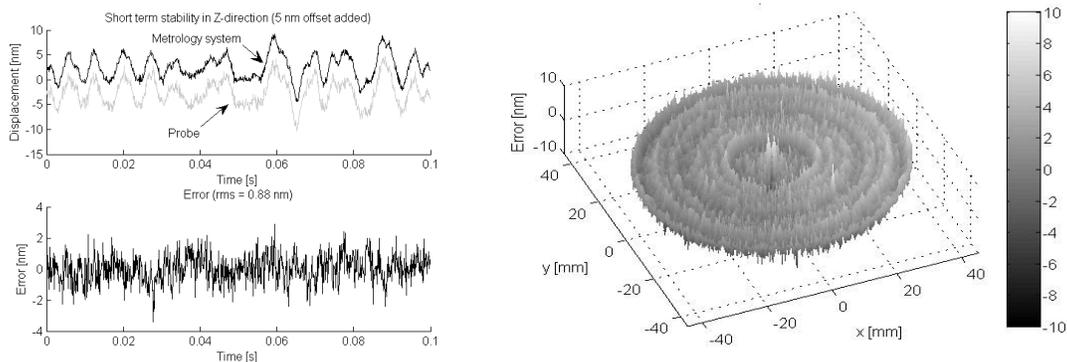
Fig. 4. Noise level at standstill, and typical repeatability for  $\varnothing 100$  mm tilted flat
