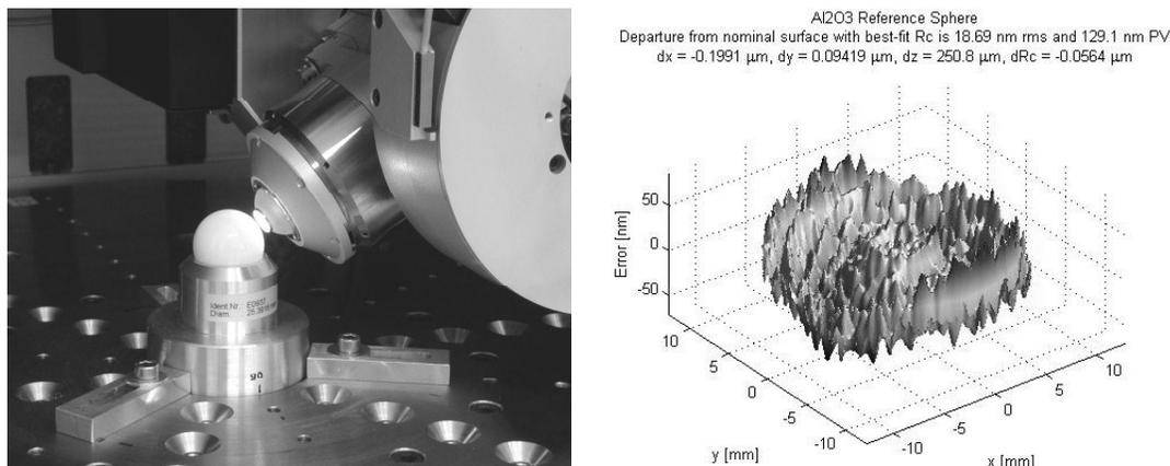
Fig. 5. Measurement result of an  $\text{Al}_2\text{O}_3$  reference sphere
