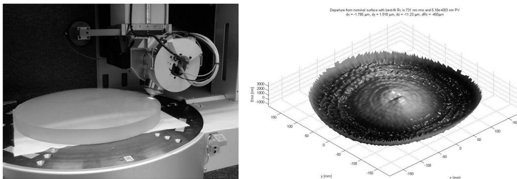
Fig. 7.  $\varnothing 380$  mm convex aspherical lens measurement (320  $\mu\text{m}$  departure from base radius)
