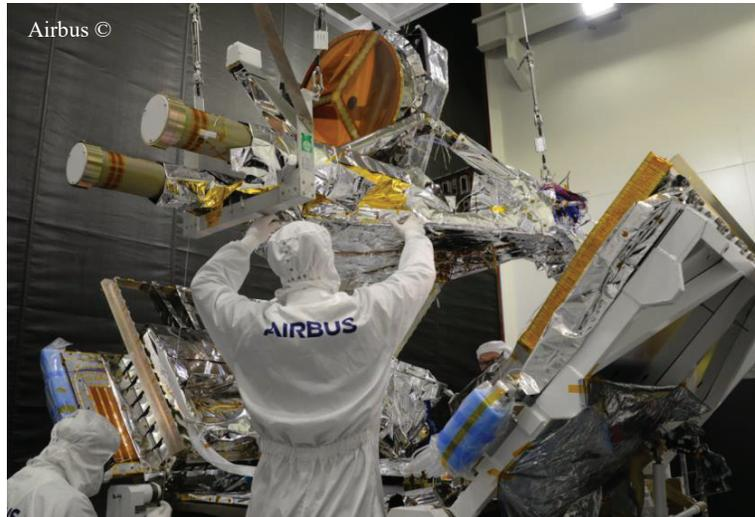
Figure 3. ATLID final coupling of OFM (top, assembly with RxA telescope and two TxA emission baffles), together with Electrical Flight Model (open structure with electronic units attached to the walls).
