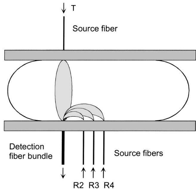
**Fig. 1** Picture showing the measurement geometry. R2, R3, and R4 denotes the reflectance modes for  $\rho=2, 3,$  and  $4$  cm, respectively. T denotes the transmittance measurement. The sampling volumes of the propagating light are schematically depicted for each case.
