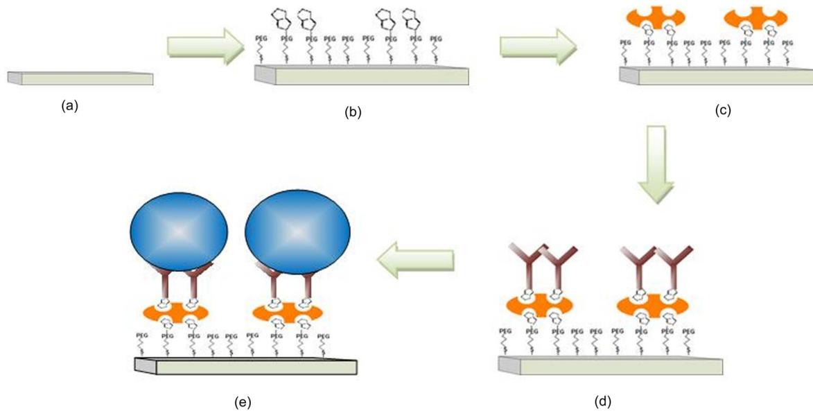
**Fig. 2** Schematic illustration of the biofunctionalization steps applied for the immobilization of the influenza A virus on GaAs (001) substrate (a) that having been etched with  $\text{NH}_4\text{OH}$  was passivated using a 2 mM solution of mixed PEG thiols (1:15) (b) and incubated in a solution of neutravidin (c). Biotinylated antibodies against influenza A were immobilized on the neutravidin-coated substrate (d), which enabled immobilizing virus particles from a solution (e).
