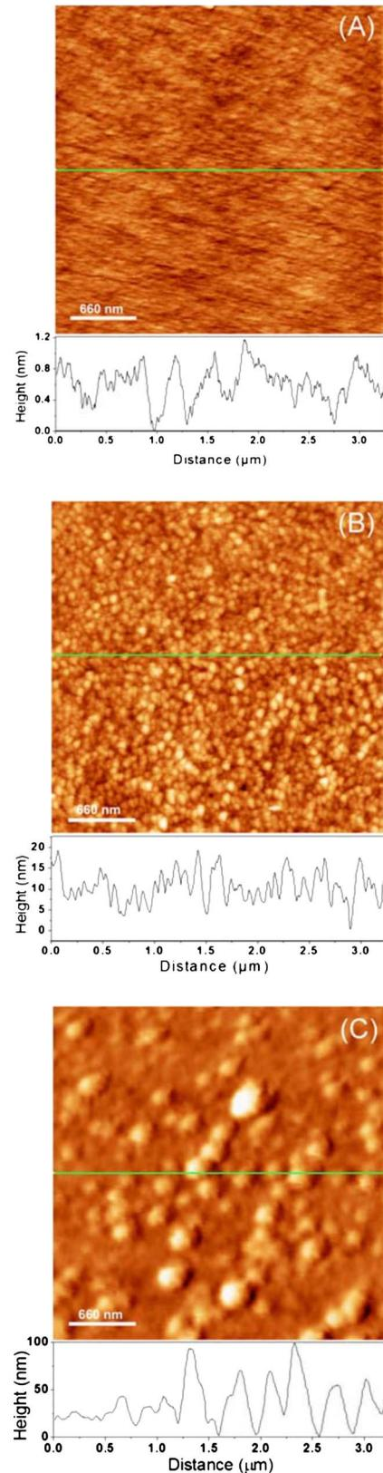
**Fig. 4** AFM images and cross-sectional scans of (a) a reference GaAs (001) sample, (b) the GaAs (001) sample biofunctionalized with PEG thiols and neutravidin, and (c) the sample that following the functionalization with the influenza A antibody was exposed to a solution of inactivated influenza A virus.
